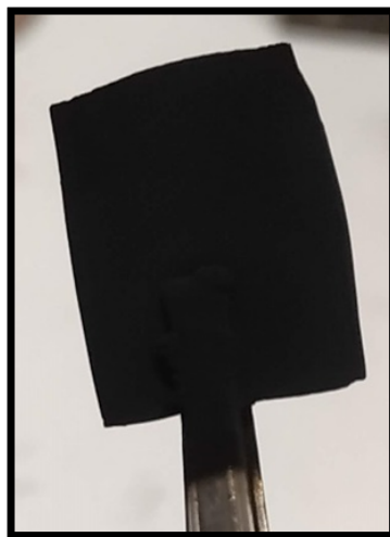
Figure 3.21: Lab-made blackbody source using soot deposited on a glass slide and heated up to 200°C using a flat resistive element underneath.
