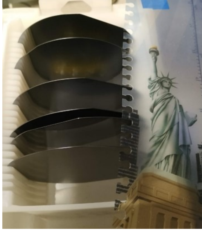
Figure 3.13: Single side polished Silicon wafer diffusers of thickness 250 \mu\text{m} and diameter 10 cm (with a measuring ruler alongside for scale)
