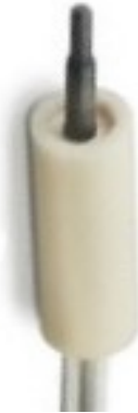
Figure 3.28: Scitec IR-Si 253 Silicon Nitride ( \text{Si}_3\text{N}_4 ) globar source that can be operated up to a maximum temperature of 1170°C [232].
