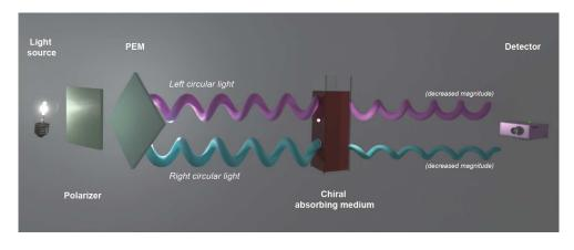
FIGURE 1.13: Schematic diagram displaying the conceptual relationships of the typical subsystems found in a CD spectrometer.
