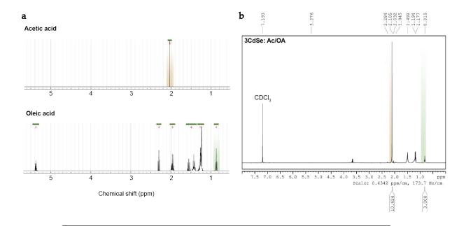
FIGURE 2.2: Simulated <sup>1</sup>H NMR spectra of (a) acetic and oleic acids, along with (b) an experimentally obtained one for carboxylates-capped 3 MLs CdSe NPLs where deuterated chloroform is used as solvent. The contributions originating from acetates (resp. oleates) are highlighted in orange (resp. green).
