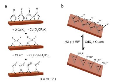
FIGURE 3.17: (a) Presumed pathway for the stages of ligand exchange carried out on zinc blende CdSe NPLs. *R* (resp. *R'* and *R''*) represents the rest of the carbon chains of acetates (resp. oleates and oleylamine). (b) Reversible back-exchange procedure, beginning from an achiral mix of carboxylates to halides co-stabilized by oleylamine, then reverting back to (*S*)-(+)-ibuprofen. Adapted from [211].
