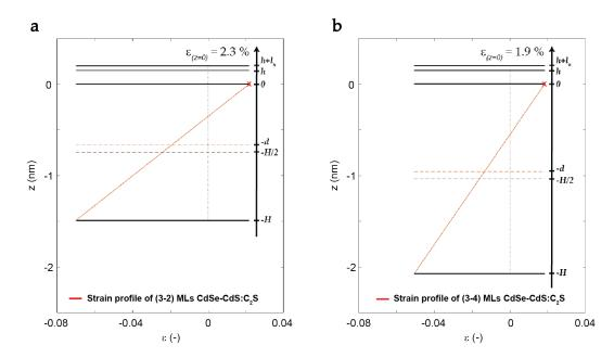
FIGURE 2.15: Strain profiles of a piece of (a) (3-2) and (b) (3-4) MLs CdSe-CdS NPL, plotted as a function of any position across its thickness direction  $\vec{z}$ . The represented surface ligands' chain length is equivalent to that of ethanethiolates, where n=2. The inlet scale corresponds to the one used to derive our three-layers model, while the *y*-axis shows a real associated unity in nm.
