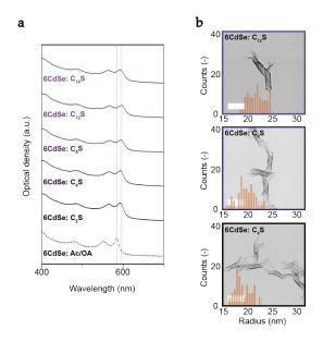
FIGURE C.4: (a) Absorption spectra of 6 MLs CdSe nanohelices before and after surface ligands modification, from initially acetates/oleates-capped to linear alkanethiolates-capped, where n = 2, 4, 8, 12, 18. Their corresponding TEM images are shown in (b). Scale bar: 200 nm.
