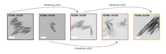
FIGURE 2.3: TEM images of as-synthesized carboxylates-capped CdSe NPLs. Nanohelices which possess an odd (resp. even) number of MLs, are subsequently obtained via the route of c-ALD with 3 (resp. 4 MLs) ones as the starting blocks. Scale bar: 200 nm.
