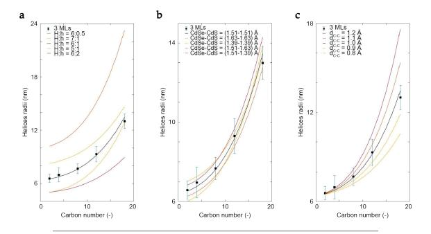
FIGURE 2.18: (a) Calculated helices radii for various ratios of H to h, where H=(ix1.51) Å, with i=5, 6, 7 and h=(jx1.51) Å, with j=0.5, 1, 2. The values of i:j are given in the inset. Other parameters are such,  $\Delta \epsilon=-21$  %,  $\Delta \epsilon''=0$  %,  $E_s=40$  GPa,  $E_d=46$  GPa,  $E_l=0.9$  GPa and  $E_l=0.9$  GPa,  $E_l=0.9$  GPa.
