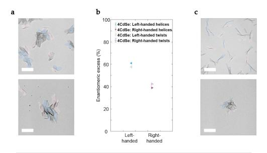
FIGURE 3.5: TEM images of separate batches of 4 MLs CdSe (a) nanohelices and (c) twists both capped by achiral carboxylates upon synthesis. The different enantiomers: left- and right-handed ones are respectively color-coded with blue and pink to ease evaluations of enantiomeric excess. Data plotted in (b) is accounted for a population of 100 objects and averaged over 3 batches of as-synthesized nanoparticles. Scale bar: 200 nm.
