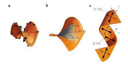
FIGURE 2.8: Scheme of a 3 MLs square nanosheet of zinc blende crystal structure. The arrows represent the compressing directions due to the adsorption of surface ligands. On the top (resp. bottom) facet, the induced stress is directed along the [1 -1 0] (resp. [1 1 0]) direction. If a wide strip ( $\tilde{w} \gg 1$ ) were to be cut from the gray zone in the middle of the nanosheet, this would result in a helix at the equilibrium state.
