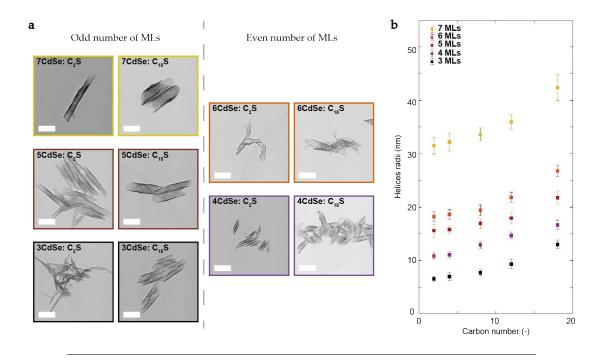
FIGURE 2.5: (a) TEM images of CdSe NPLs which have been chemically surface-modified and present either ethanethiolates or octadecanethiolates on their outer surface. Left (resp. right) panel displays images of odd (resp. even) number of MLs NPLs. Scale bar: 200 nm. (b) Experimental helices' radii deduced from the analysis of microscope images for CdSe NPLs with thicknesses ranging from 3 to 7 MLs, averaged over a population of 100 nanohelices.
