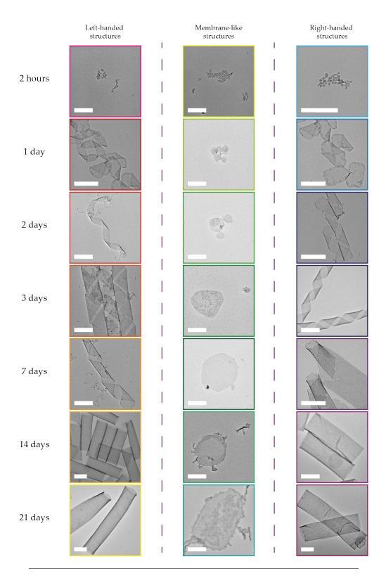
FIGURE 4.2: TEM images of the kinetic shape transition of gemini surfactant assemblies upon silica coating, where the molecules are beforehand complexed by (left column) D-(+)-, (middle column) DL- and (right column) L-(-)- malate ions. Scale bar: 500 nm.
