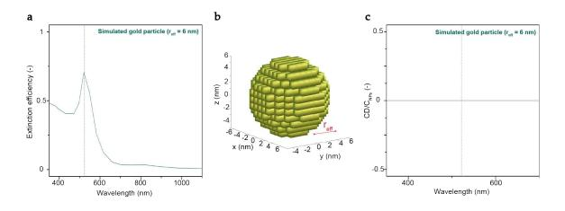
FIGURE 4.14: (a) Simulated extinction spectrum of a single isolated gold nanoparticle, with a radius  $r_{eff}=6$  nm suspended in water. (b) Schematic of a spherical object generated under discrete dipole approximation. (c) Computed CD trend as the extinction difference under left- and right-handed circularly polarized light excitations.
