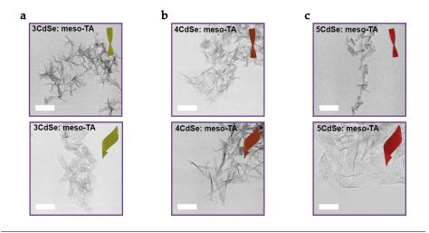
FIGURE D.1: TEM images of two different lateral sizes of 3 (resp. 4 and 5 MLs) CdSe NPLs capped by *meso*-tartaric acid molecules, as displayed in (a) (resp. (b) and (c)). Scale bar: 200 nm.
