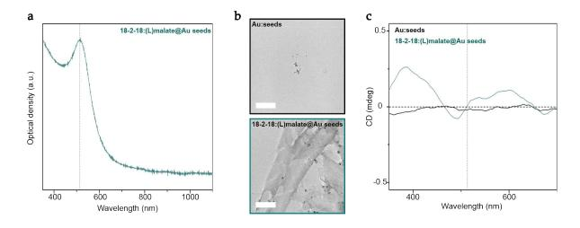
FIGURE 4.8: (a) Absorption spectra of *18-2-18*:(*L*)malate@Au seeds in distilled water. (b) TEM images of the (top) pre-prepared gold seeds and (bottom) tribrid surfactant-silica-gold seeds structures. Scale bar: 200 nm. (c) CD spectra of these two corresponding solutions in distilled water. The dashed lines indicate the peak of plasmonic resonance at 513 nm.
