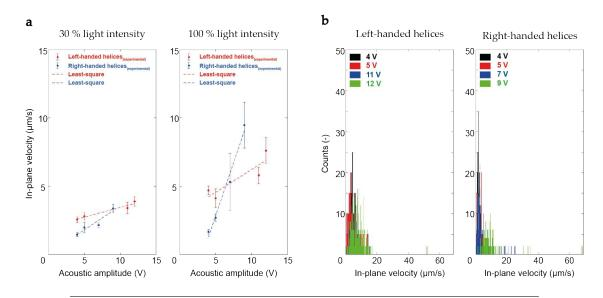
FIGURE 4.22: (a) Average in-plane velocity of 18-2-18:(D/L)malate@FITC left-and right-handed silica helices as a function of acoustic amplitudes, under two different illuminated light intensities at 488 nm. During experiment, the acoustic frequency is set at 1.88 MHz. (b) Histogram plots for the tracked fluorescent particles of opposite handedness, illuminated at 100 % of light intensity. In each case, a total number of more than 50 particles is accounted for. Bin:  $0.2 \ \mu m \cdot s^{-1}$ .
