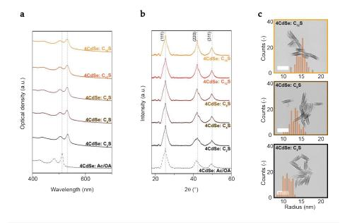
FIGURE C.2: (a) Absorption spectra of 4 MLs CdSe nanohelices before and after surface ligands modification, from initially acetates/oleates-capped to linear alkanethiolates-capped, where n = 2, 4, 8, 12, 18. Their corresponding X-ray diffractogrammes (resp. TEM images) are shown in (b) (resp. (c)). Scale bar: 200 nm.
