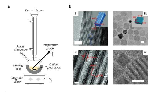
FIGURE 1.8: (a) Scheme of a three-neck flask mounted onto a heating and stirring device adapted for the synthesis of colloidal nanoparticles. (b) TEM and HRTEM images of (i, ii) hexagonal wurtzite CdSe nanoribbons. Scale: 20 and 2 nm. Whereas in (iii, iv), cubic zinc blende CdSe NPLs are shown. Scale: 10 nm. Adapted from [10, 11].
