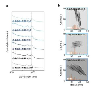
FIGURE C.8: (a) Absorption spectra of (3-4) MLs CdSe-CdS nanohelices before and after exchanges of surface ligands, from initially acetates/oleates-capped to linear alkanethiolates-capped, where n = 2, 4, 8 12, 18. Their corresponding TEM images are shown in (b). Scale bar: 200 nm.
