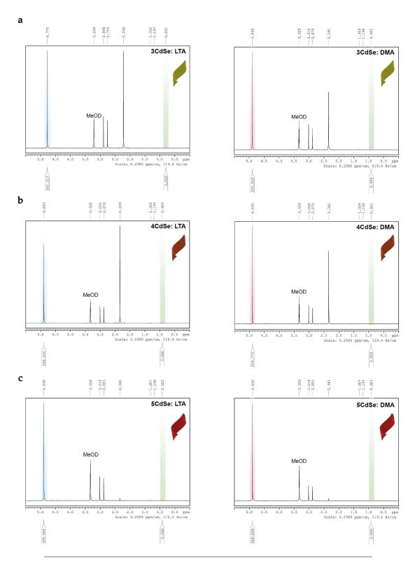
FIGURE D.5:  $^{1}$ H NMR spectra of L-(+)-tartrate (resp. D-(+)-malate) functionalization displayed in left (resp. right) panel, for NPLs that are (a) 3, (b) 4 and (c) 5 MLs thick. Highlighted areas in cyan (resp. magenta) correspond to the characteristic resonance of L-(+)-tartaric acid (resp. D-(+)-malic acid), while the green ones represent the methyl contribution from oleates.
