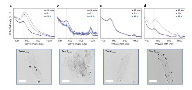
FIGURE 4.10: Absorption spectra (top panel) and TEM images (bottom panel) of the associated *18-2-18:(L)*malate@Au grown seeds, under the conditions presented in Tab. 4.3. The dashed lines indicate the shift of the resonance peak gradually to 558 and 549 nm in cases of tests A and D respectively, while being stucked at 513 nm in both tests B and C. Scale bar: 200 nm.
