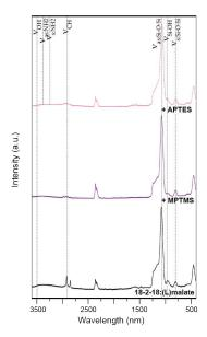
FIGURE 4.6: FTIR spectra of (black) the resulted 18-2-18:(L)malate silica helices prior to any surface chemical alterations, then either (violet) thiolmodified with MPTMS or (pink) amino-modified with APTES.
