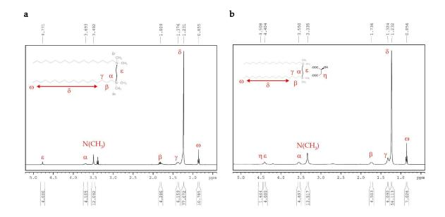
FIGURE 4.1:  $^{1}$ H NMR analysis of (a) the as-synthesized  $^{18-2-18}$ :bromide gemini surfactant molecule and (b)  $^{18-2-18}$ :( $^{1}$ L)malate after counterion exchanges. Estimated values for the proton assessment: 0.9 ppm (6H, CH $_3$  x2); 1.2 ppm (56H, (CH $_2$ ) $_{14}$  x2); 1.3 ppm (4H, CH $_2$  x2); 1.7 ppm (4H, CH $_2$  x2); 3.3 ppm (12H, N $^+$ (CH $_3$ ) $_2$  x2); 3.6 ppm (4H, CH $_2$  x2); 4.3 ppm (4H, N $^+$ (CH $_2$ ) $_2$ N $^+$ ); 4.5 ppm (2H, CH x2).
