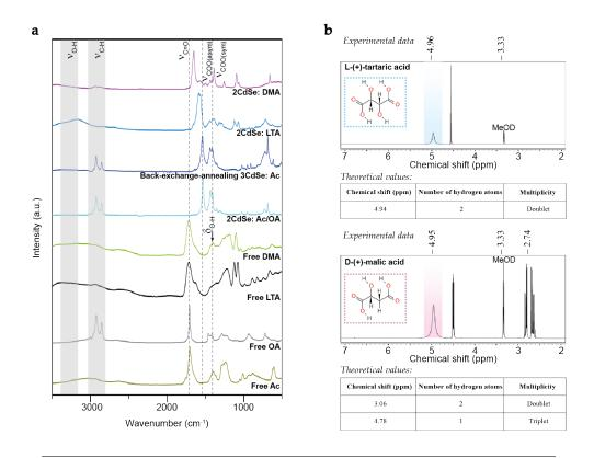
FIGURE 3.14: (a) FTIR spectra of free carboxylic acids and carboxylates-bound CdSe NPLs. (b) Experimental and theoretical  $^{1}$ H NMR findings of L-(+)-tartaric and D-(+)-malic acids, where deuterated methanol is used as the solvent.
