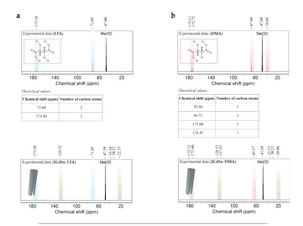
FIGURE D.4: (a) Experimental and theoretical  $^{13}$ C NMR findings of L-(+)-tartaric and D-(+)-malic acids, where deuterated methanol is used as the solvent. Bottom panel displays the experimental spectra of large 2 MLs CdSe nanoscrolls that have been subjected to these ligand exchanges, with slight traces (color-coded in green) from oleic acid.
