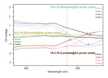
FIGURE 4.13: CD spectra of the associated 18-2-18:(D/DL/L)malate@Au grown seeds, synthesized under the conditions presented in Fig. 4.12. Red marks indicate the crossing wavelength for each pair of bisignated patterns, where the same amount of gold seeds is employed. The dashed lines indicate the peak of plasmonic resonance at 558 nm.
