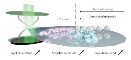
FIGURE 5.3: Manipulating fluorescently labeled silica objects under simultaneous opto- and acousto-perturbations. The above cartoon displays the enhanced-aggregation phenomenon of particles in a cavity's mid-plane, at an average in-plane velocity that increases with both the magnitude of light and acoustic excitations.
