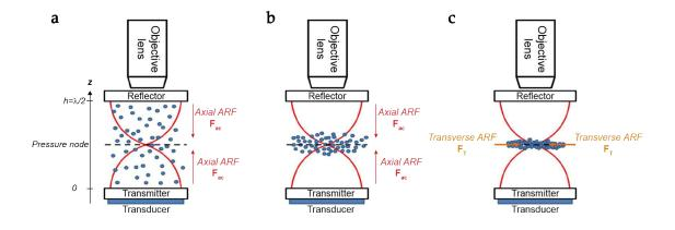
FIGURE 1.19: Scheme of a suspension of particles subjected to ARF manipulation over time. (a,b) The primary axial force  $\mathbf{F}_{ac}$  drives the objects toward the resonant cavity's mid-height and confines them in the nodal plane. (c) The transverse force  $\mathbf{F}_T$  then contributes to further compacting these latter into forming an aggregate. Adapted from [136].
