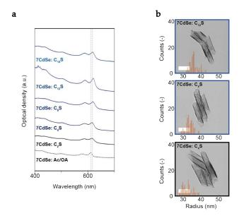
FIGURE C.5: (a) Absorption spectra of 7 MLs CdSe nanohelices before and after surface ligands modification, from initially acetates/oleates-capped to linear alkanethiolates-capped, where n = 2, 4, 8, 12, 18. Their corresponding TEM images are shown in (b). Scale bar: 200 nm.
