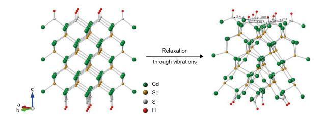
FIGURE 2.10: Relaxation of a tiny piece of 4 MLs NPL capped with bisulfides, possessing the chemical formula  ${\rm HS^-}$ . It demonstrates that the sulfide-to-sulfide distance is reduced compared to the case of a zinc blende CdS bulk, where its lattice parameter equals 4.11 Å.
