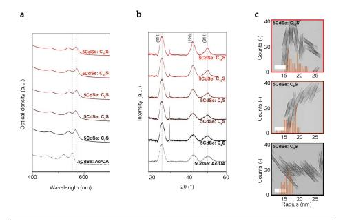
FIGURE C.3: (a) Absorption spectra of 5 MLs CdSe nanohelices before and after surface ligands modification, from initially acetates/oleates-capped to linear alkanethiolates-capped, where n = 2, 4, 8, 12, 18. Their corresponding X-ray diffractogrammes (resp. TEM images) are shown in (b) (resp. (c)). Scale bar: 200 nm.
