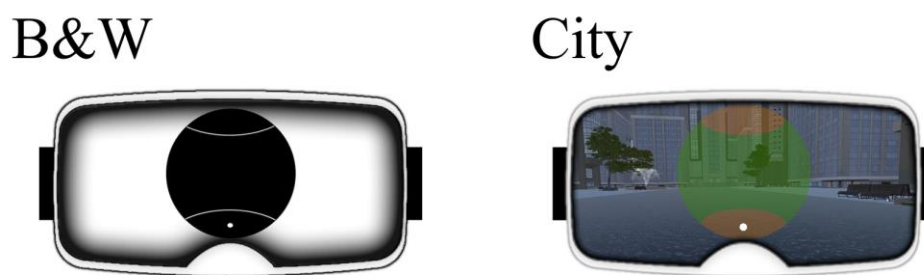
Figure 4.22. HMD Visual display. Subjects perceived a 3-dimensional hand position displayed through a VR headset screen in B&W and City environment.
