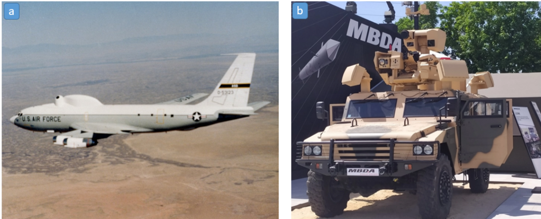
Figure 1.2: Illustration of a laser system: (a) left-side view of an NKC-135 airborne laser [1] and (b) MBDA showcased HELMA-P laser anti-drone system mounted on an Arqus Sherpa armored vehicle [2].
