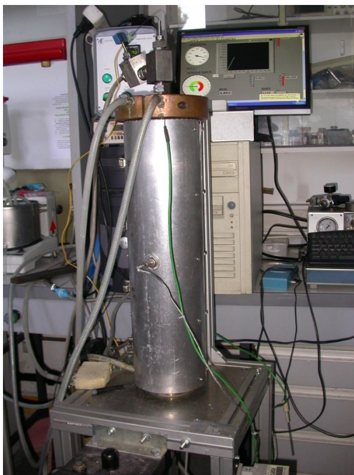
Figure 2-3. Autoclave artisanal de polymérisation HT/HP.
