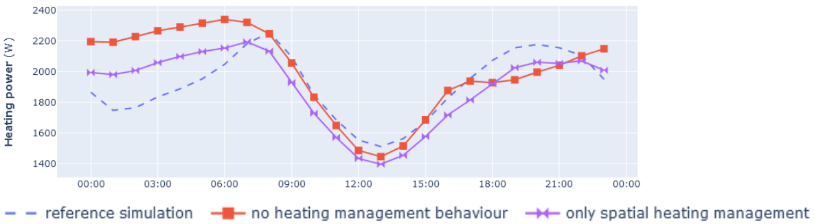
Figure 5. Comparison between heating power of reference simulation, absence of heating management and spatial heating management.
