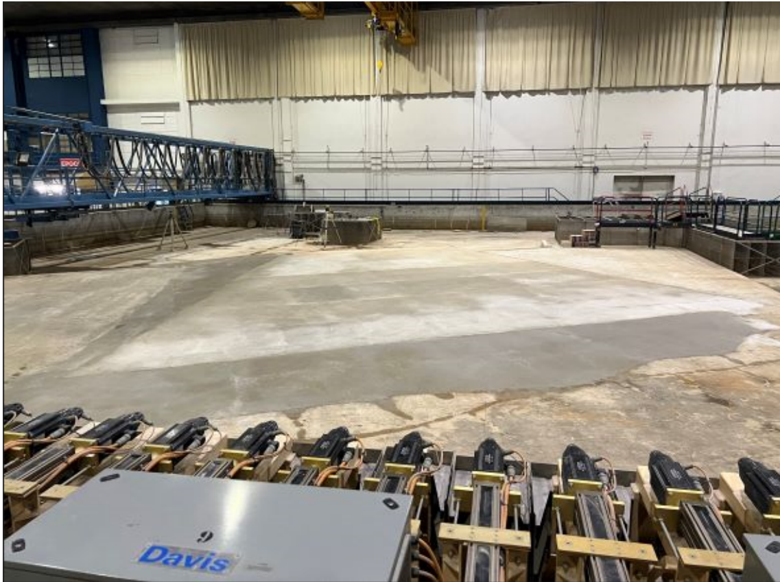
Figure 5.4: The constructed bathymetry as part of 3DWaveBI, in the wave tank at Chatou. Wave-maker paddles can be seen at the bottom of the picture.
