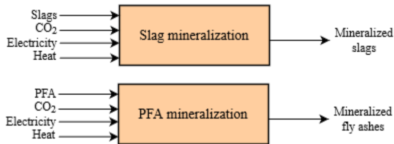
Figure 33: Input/output flows in CO 2 mineralization processes.
