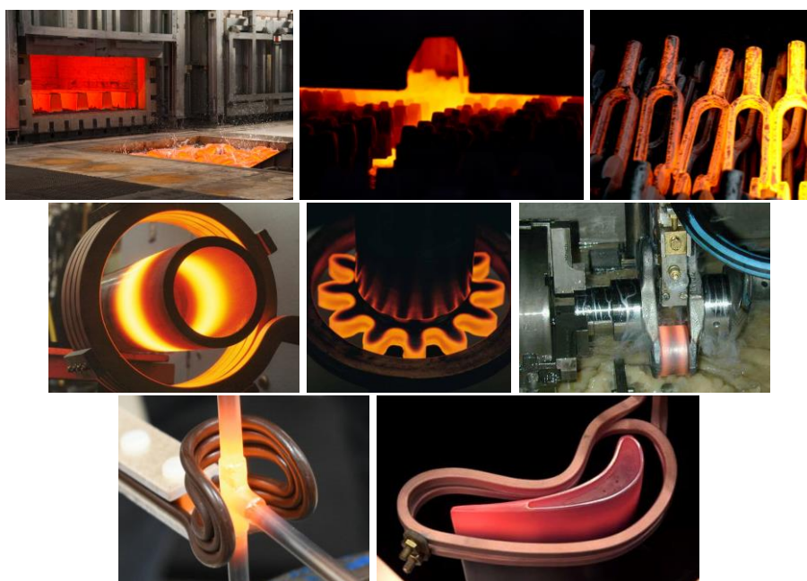
Fig. 1.2 Some induction heating industrial applications.
