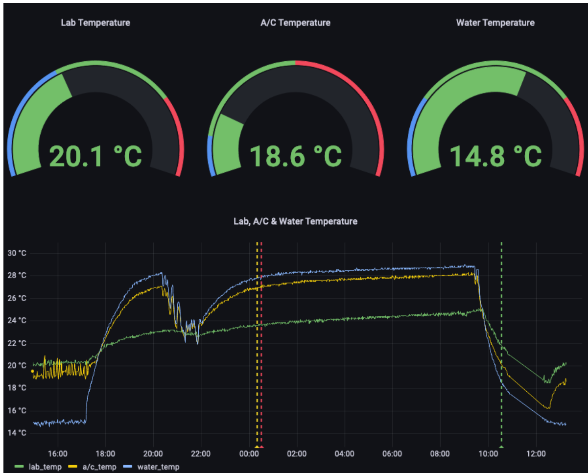
Figure 2.12 – Experiment monitoring GUI. The Grafana interface for the experiment monitoring system can be accessed locally or from outside the lab via a VPN. Gauges and time series plots indicate the current state of affairs of connected lab equipment, with the vertical lines corresponding to situations that trigger an automatic alert, here in the case of a lab-wide A/C failure. The limit for the lab temperature is passed at the yellow line, and after not falling below the limit in terms of its average value for a pre-set duration, an alert message is sent (red line). When the situation is back to normal, another e-mail is sent to inform the users (green line).
