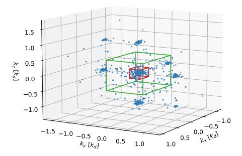
**Figure 5.8 – Measurement volume for condensate fluctuations.** Same 3D momentum distribution as shown in fig. 3.2, with the different measurement volumes highlighted. The BEC atom number is evaluated by counting the atoms in the o-th order diffraction peak in a cube of size  $0.3\ k_d$  (red). It is set into relation with the condensed fraction not via comparison with the total atom number, but the atom number in the FBZ only (green).
