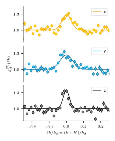
Figure 3.3 – Anomalous correlations revealing pairs of atoms at opposite momenta. One-dimensional cross-sections of  $g_A^{(2)}(\delta {\bf k})$  are taken along the three lattice axes, with transverse integration using  $\delta k_\perp = 3.0 \times 10^{-2} \ k_d$  and a longitudinal voxel size of  $\delta k_\parallel = 1.2 \times 10^{-2} \ k_d$ . Gaussian functions (solid lines) are used to fit the data, and error bars are determined from the inverse square root of the voxel count.
