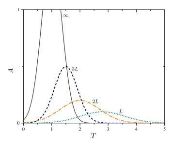
**Figure 5.2 – Finite size scaling.** Behavior of a physical observable A in the vicinity of the critical point  $T_c=1$  as a function of temperature T for different system sizes L. As L increases, the position and shape of the peak is shifted towards the divergence situation found for  $L \to \infty$ . Taken from [206].
