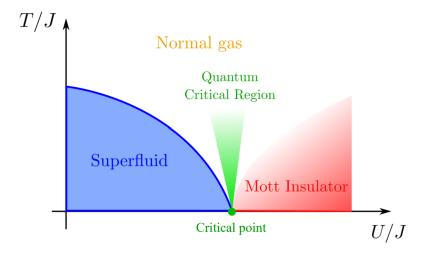
**Figure 2.9 – Bose-Hubbard phase diagram.** Temperature rescaled by the tunnel coupling as a function of the BH parameters u=U/J. The quantum phase transition is located on the x-axis. At finite T the superfluid and Mott insulating phases are separated by a normal gas phase. Above the quantum critical point there is a region where quantum critical phenomena can still be expected to be observable despite the finite temperature. Taken from [53].
