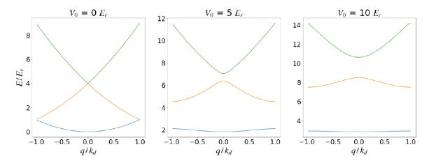
Figure 2.4 – Dispersion relations of the lowest three Bloch bands for increasing lattice amplitudes  $V_0$ . The mean energy of the band grows with the band index. In 3D a gap opens up between the first two bands at the edge of the FBZ for  $V_0 \gtrsim 2.2$ . Taken from [53].
