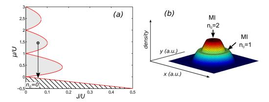
**Figure 2.7 – Phase diagram (a) and spatial density profile (b) for the inhomogeneous system.** (a) The phase diagram (chemical potential as a function of the tunnel coupling, both in units of the on-site interaction) shows the appearance of Mott insulating shells at integer filling. (b) In the inhomogeneous system a wedding-cake structure is formed with Mott shells surrounded by superfluid shells. Taken from [92].
