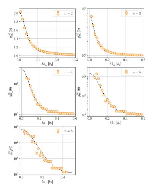
Figure 4.5 – Effect of the transverse integration  $\delta k_{\perp}$  on the amplitudes of the correlation functions  $g_{\delta k_{\perp}}^{(n)}$ . Varying  $\delta k_{\perp}$  while keeping the longitudinal dimension of  $V_{\Omega}$  at a constant  $\delta k=1.5\times 10^{-2}k_d \leq l_c$  allows for the extrapolation of the fully contrasted correlation functions  $g^{(n)}$  in the limit  $\delta k_{\perp} \to 0$  (black dashed lines).
