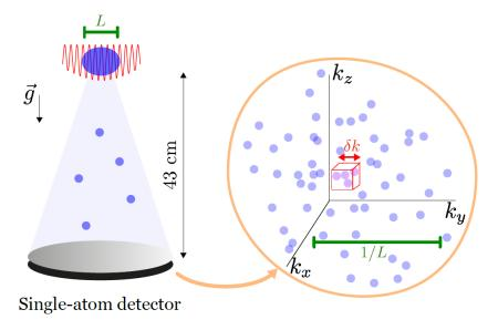
Figure 4.1 – Schematic representation of the FCS measurement. The 3D momentum distribution is recorded in the far field after a long free fall from the optical lattice. The measurement volume  $V_{\Omega}=(\delta k)^3$  has to be chosen to be smaller than the size of a single mode in momentum space  $V_c=(2\pi/L)^3$ .
