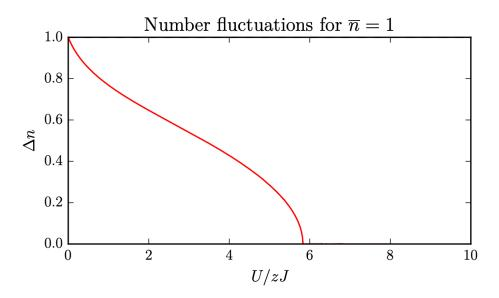
Figure 5.6 – Onsite number fluctuation across the superfluid to Mott insulator phase transition. Contrary to the condensate number fluctuations  $N_0$ , the onsite fluctuations vanish upon approaching the phase transition but remain large in the superfluid region due to the long-wavelength coherence of the condensate wavefunction. Taken from [223].
