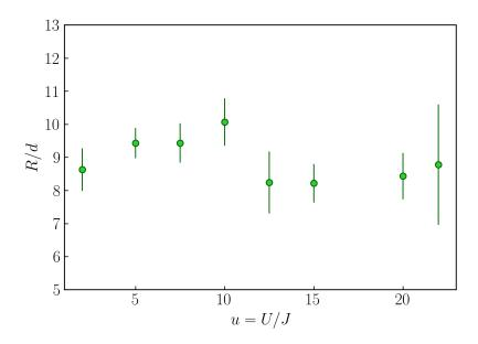
**Figure B.1 – In-situ cloud size as a function of interactions.** Vertical error bars are one standard deviation on extracted in-situ sizes. The extracted values show no systematic tendency as a function of U/J an are therefore taken to be constant.
