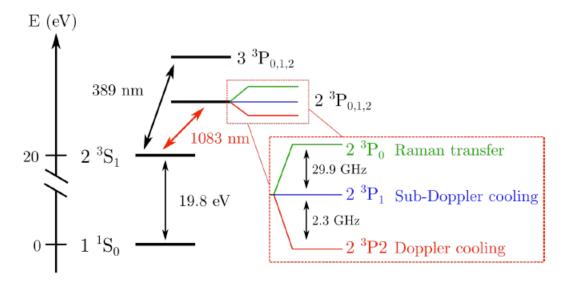
**Figure 2.1 – Relevant energy levels of** <sup>4</sup>**He.** The metastable state 2  $^3$ S<sub>1</sub> is the starting point for all cooling, trapping and imaging transitions towards the 2  $^3$ P<sub>0,1,2</sub> states, which can be accessed with standard near-infrared lasers at wavelengths around 1 $\mu$ m. Taken from [52].
