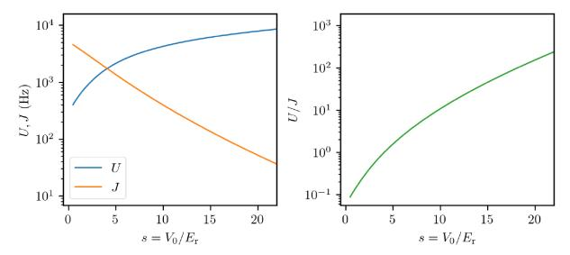
Figure 2.6 – Evolution of the Bose-Hubbard energy terms (a) and their ratio (b) with the lattice amplitude. From figure (a) it is clear that with the lattice amplitude (expressed here in units of the recoil energy) as only tunable parameter, the two energy terms J and U of (2.19) are not independent. Their ratio (b) is what determines the macroscopic state of the ground state. Taken from [52].
