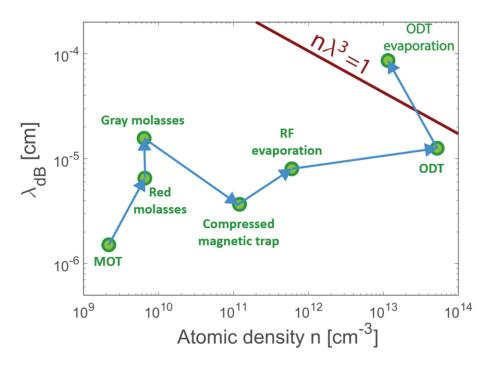
Figure 2.3 – Phase-space density at the different stages of the cooling sequence. A sequence of different cooling techniques has to be employed in order to be able to cross the quantum degeneracy limit of  $\lambda_{\rm dB}^3$  n=1. Taken from [53].
