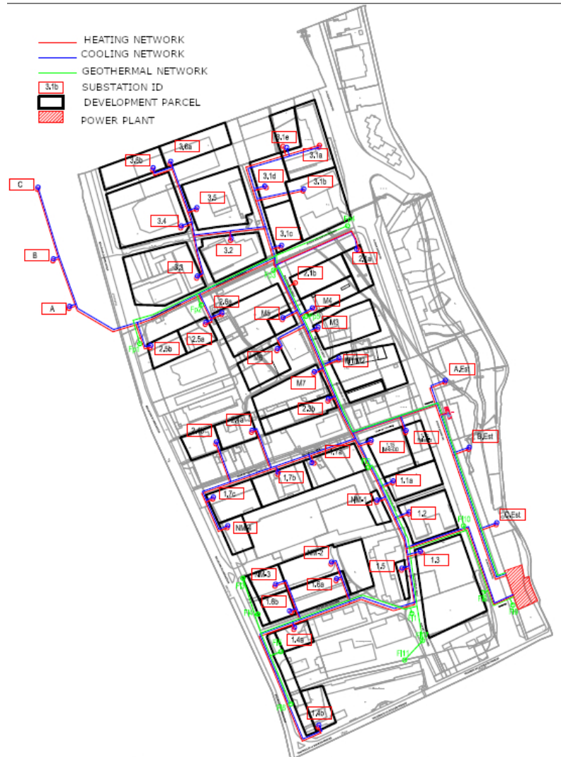
Figure 6.5: Layout of the geothermal heating and cooling network of the MSE eco-district illustrating the locations of substations. Each substation ID corresponds to two substations: one for heating and one for cooling (source: Idex document).
