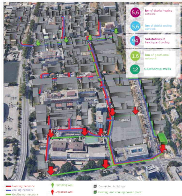
Figure 6.3: Map of the MSE eco-district showing the locations of pumping and injection geothermal wells and the heating and cooling power plant (source: Idex document).
