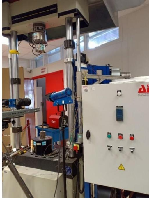
Figure 30 Machine de traction
