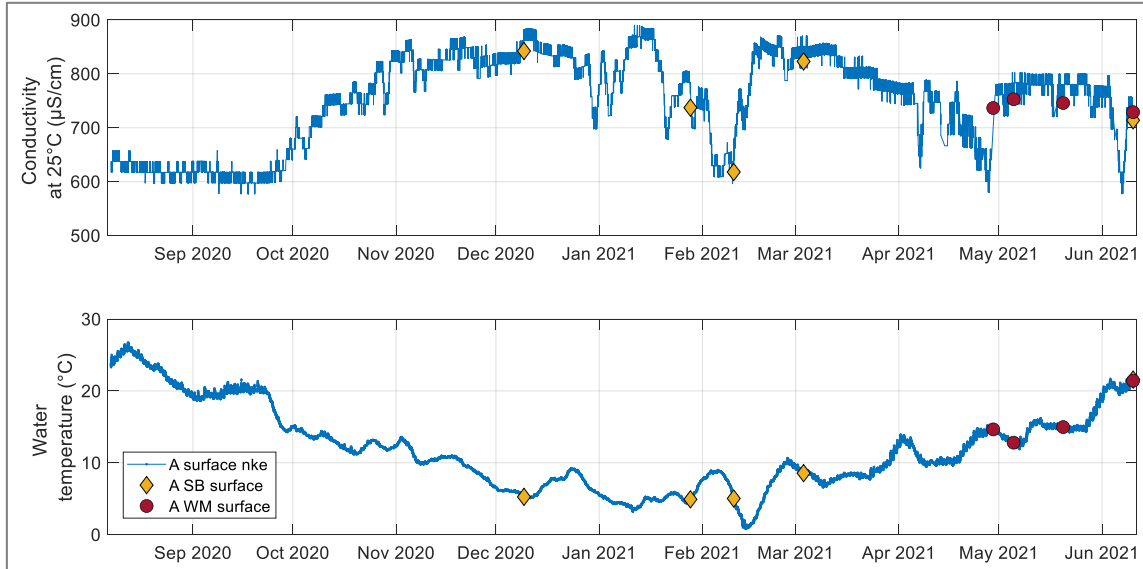
Figure A.5. Conductivity and water temperature measurement from nke sensor (continuous), and from references probes SeaBird (SB) and WiMo (WM), at point B, from 07/08/2021 to 10/06/2021.
