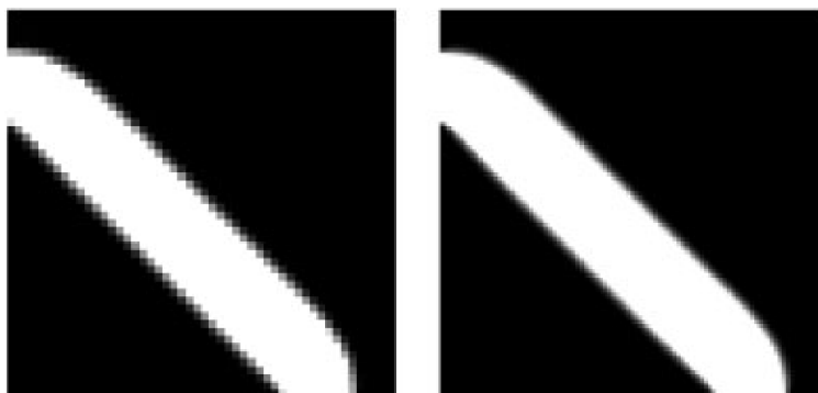
Figure 3.5: Optimal designs for the Bend Pipe problem of [79] showcasing the staircase effect. The computation was performed on regular grid type meshes of respectively 2500 (to the left) and 10000 (to the right) elements.
