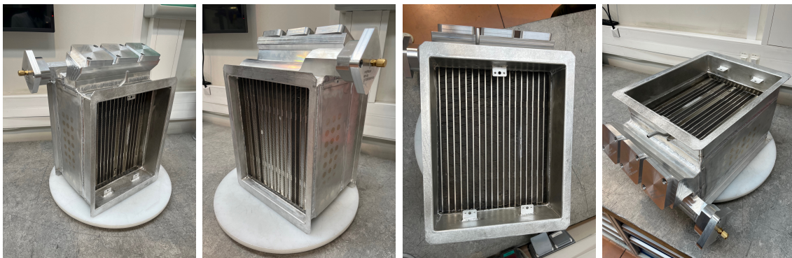
Figure 6.1: PFHE actually in service shown from different perspectives.
