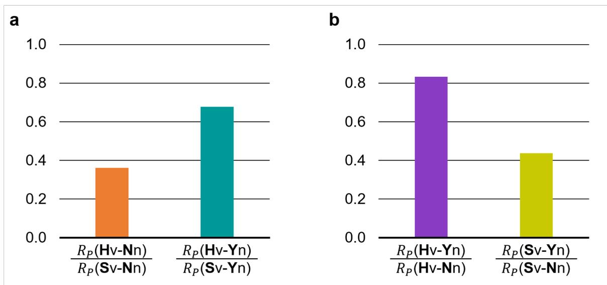
Figure 4.4-12 – Ratio of the area-normalised product resistance to mass transfer ( $R_p$ ) for dried product layer thickness ( $l_d$ ) of 5 mm between experimental conditions (a) using different vial types and (b) with and without a nucleating agent. Hv-Nn, Hv-Yn, Sv-Nn, Sv-Yn, and Sv-Nn-S are the experimental conditions described in Table 4.4-1.
