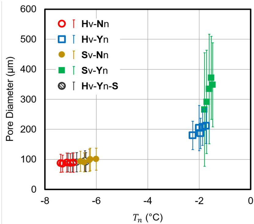
Figure 4.4-8 – Pore diameters as a function of the nucleation temperature ( $T_n$ ). Each mark represents the mean pore diameter value and  $T_n$  for a sample (repetition). Error bars represent the standard deviations.
