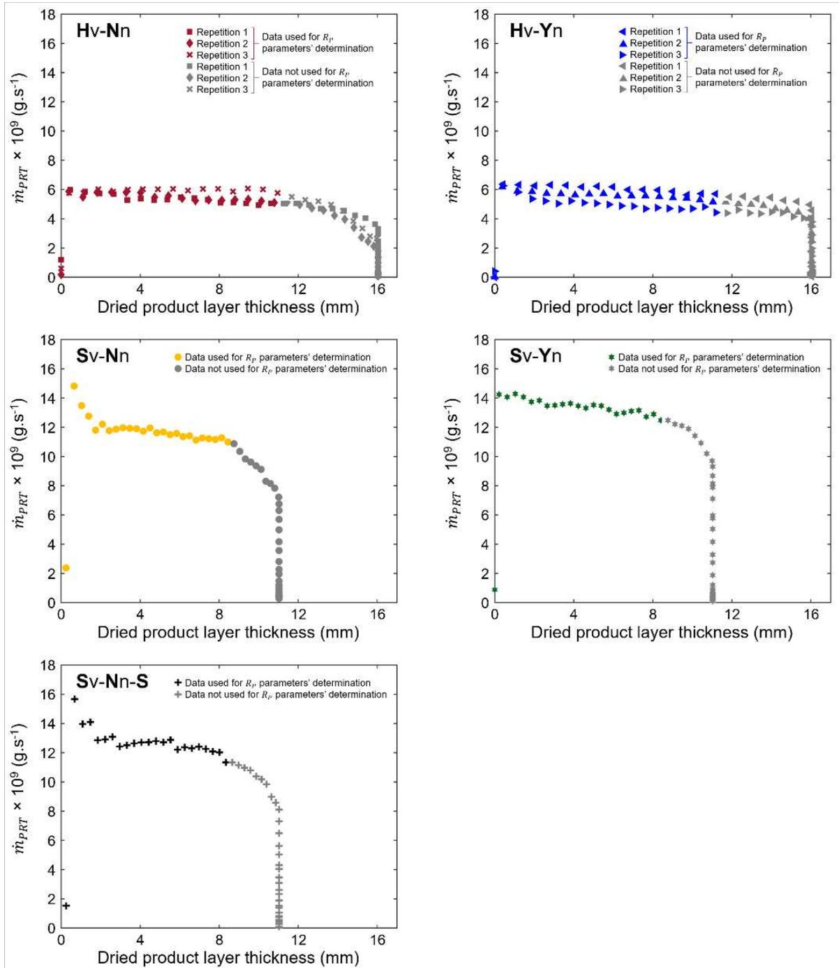
Figure 4.4-10 – Evolution of the vial-averaged mass flow rates ( $\dot{m}_{PRT}$ ) with the dried product layer thickness ( $l_d$ ). Vial-averaged  $\dot{m}_{PRT}$  values were determined by the pressure rise test method using Equation 4.4-9. Hv-Nn, Hv-Yn, Sv-Nn, Sv-Yn, and Sv-Nn-S are the experimental conditions described in Table 4.4-1.
