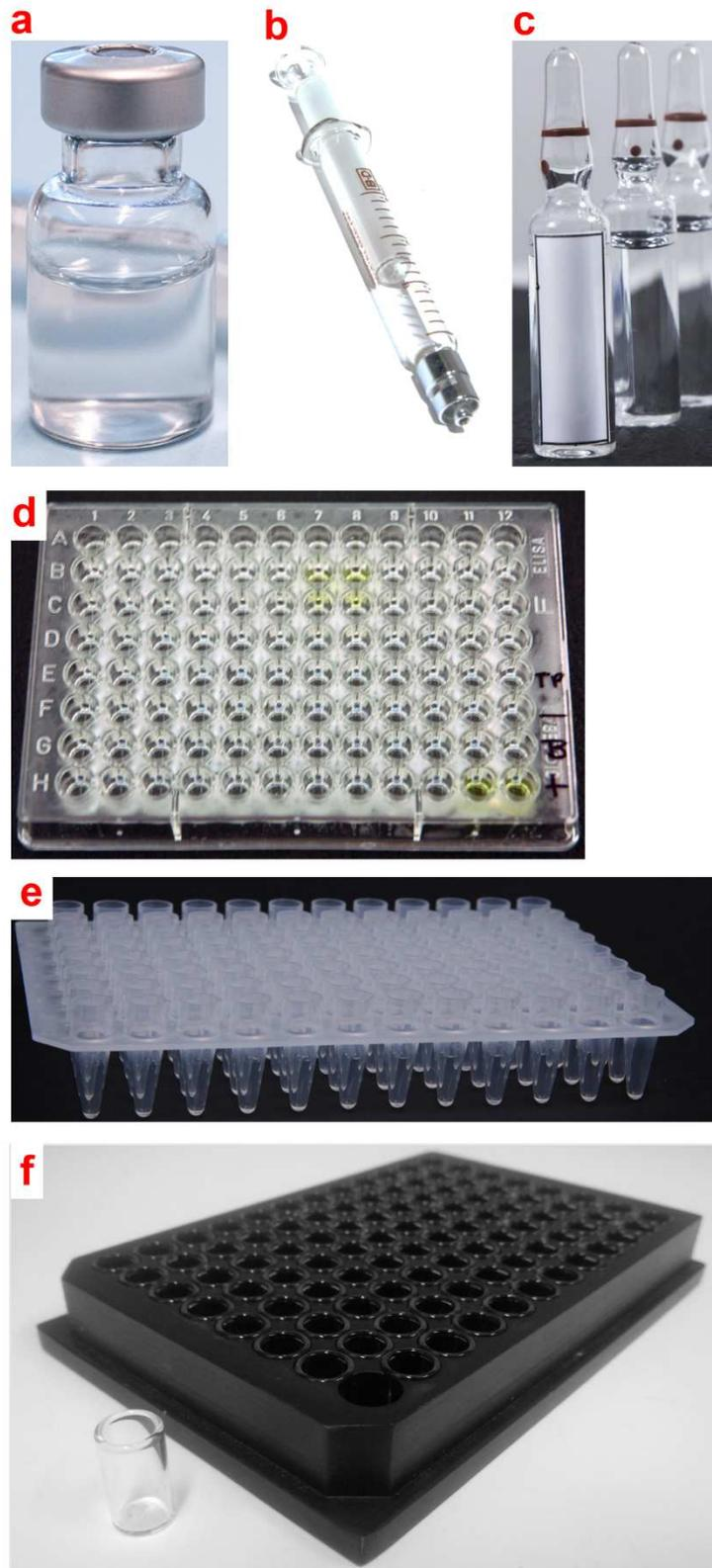
Figure 2.2-2 – Containers to perform freeze-drying. (a) Serum vial. (b) Syringe. (c) Ampoule. (d) 96-well PCR-plate. (e) Plastic 96-well plates. (f) 500- $\mu$ L high-throughput vial in front of a 96-Well Freeze-Drying System manufactured by VirTis, consisting of an aluminium well plate carrying 96 high-throughput vials.
