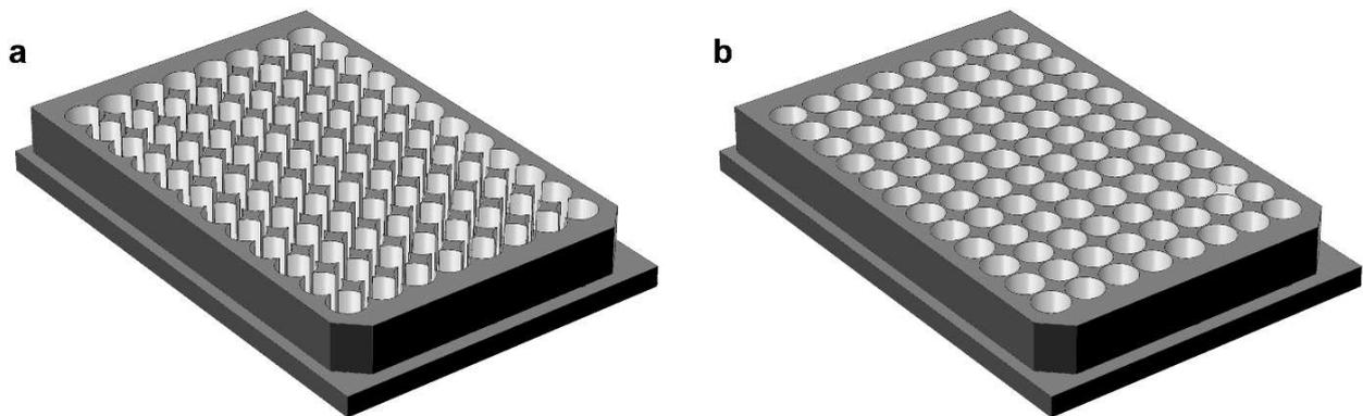
*Figure 4.2-11 – 3D reconstruction of a well plate. (a) Geometry of a “real” well plate with pillars. (b) Geometry of a simplified well plate without pillars, assuming the well diameter equal to the external vial diameter.*
