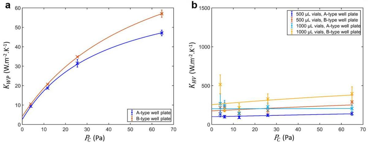
Figure 4.1-4 – Heat transfer coefficients (a) between the shelf and well plate bottom ( $K_{WP}$ ), and (b) between the well plate and vial bottom ( $K_{HV}$ ), vs. chamber pressure ( $P_C$ ). The curves correspond to the values calculated with Equation 4.1-16, Equation 4.1-17, and Equation 4.1-19 to Equation 4.1-24. Error bars represent standard deviations.
