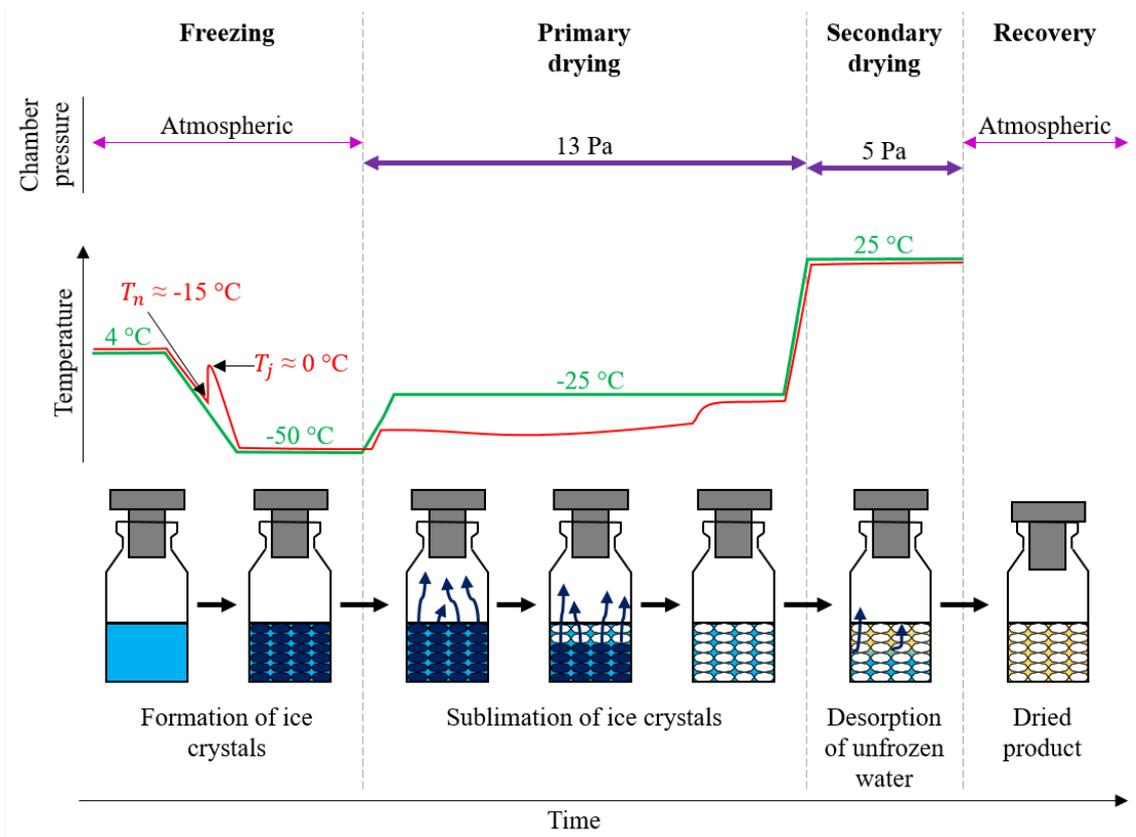
Figure 2.1-3 – Schematic illustration of the freeze-drying process. Green and red curves represent the shelf temperature and product temperature, respectively.  $T_n$  is the nucleation temperature, and  $T_j$  is the freezing-point depression temperature. Numeric values are examples of typical values. Not in scale (adapted from Kawasaki et al., 2019).
