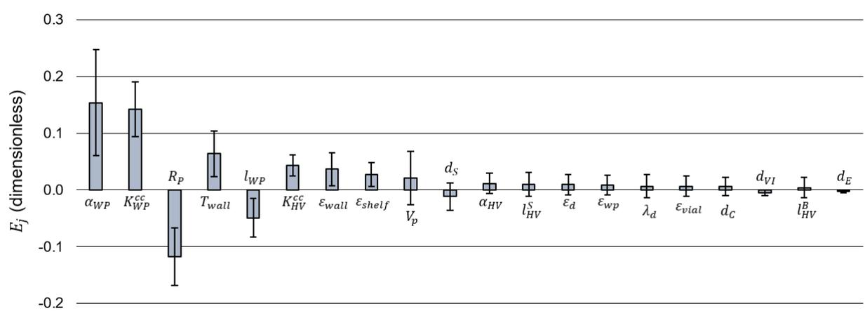
Figure 4.2-10 –  $E_j$  values of the parameters reported in Table 4.2-3, calculated using Equation 4.2-20. Grey bars represent the average values for the domain samples, and error bars represent the standard deviations within the “domain samples”.
