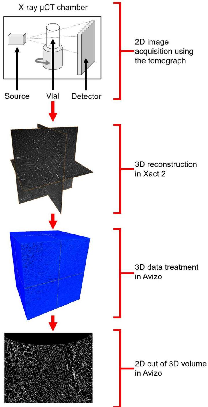
Figure 4.4-4 – Data processing scheme of the X-ray micro-computed tomography (μCT).
