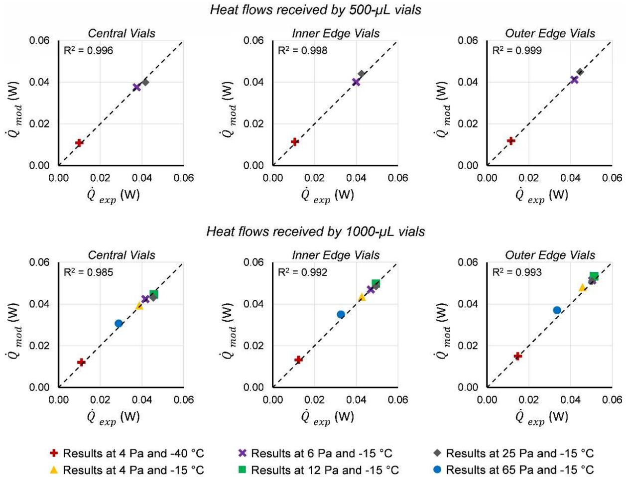
Figure 4.2-5 –  $\dot{Q}_{exp}$  vs  $\dot{Q}_{mod}$ . The 1:1 dotted line represents perfect agreement between predicted and observed values. The values of the coefficient of determination ( $R^2$ ) are reported in each graph.
