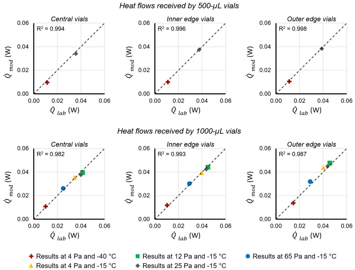
Figure 4.3-13 – Comparison of mean experimental ( $\dot{Q}_{lab}$ ) and simulated ( $\dot{Q}_{mod}$ ) heat flows received by 500-µL vials and 1000-µL vials in an A-type well plate in the centre of the shelf. Several combinations of shelf temperatures (-40 °C and -15 °C) and chamber pressures (4, 12, 25, and 65 Pa) were tested. Central vials, inner edge vials, and outer edge vials refer to positions in Figure 4.3-1. The values of the coefficient of determination (R2) are reported in the figure.
