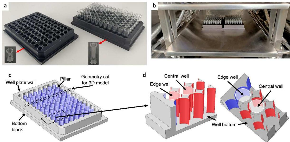
Figure 4.2-1 – Vials and well plate geometry. (a) Well plates filled with 500- $\mu\text{L}$  vials (left) and 1000- $\mu\text{L}$  vials (right). (b) Well plates and vials inside a freeze-dryer. (c) Well plate geometry with pillars coloured purple. (d) Geometry details with different view angles. Red surfaces are the pillar surfaces facing the vial. Blue surfaces are the well plate wall surfaces facing the vial.
