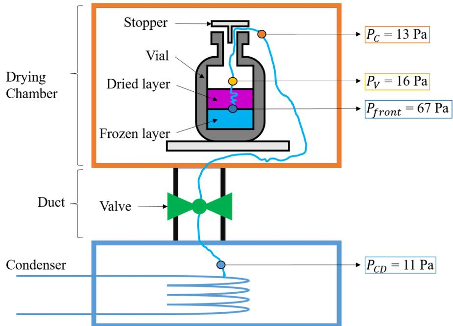
Figure 2.3-1 – Mass transfer in primary drying: schematic of resistances. Typical pressure values are given (adapted from Pikal, 1985). Note that the vapour-ice equilibrium pressure at the condenser temperature is lower than indicated, e.g. at  $-60 \text{ }^\circ\text{C}$  it would be  $1.1 \text{ Pa}$ .
