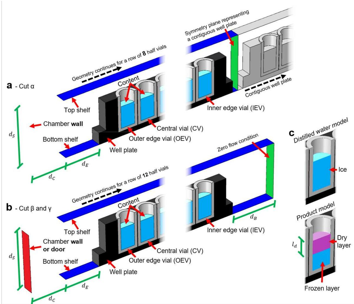
Figure 4.3-2 – Model geometry (not in scale) for 500- $\mu$ L vials in well plates (a) in the centre of the shelf (cut  $\alpha$  in Figure 4.3-1), and (b) near the chamber door or wall (cut  $\beta$  or  $\gamma$  in Figure 4.3-1). Overall view, with only the vials closer to the edge represented for clarity. (c) Detail of the vial and its content for the distilled water model and product model.
