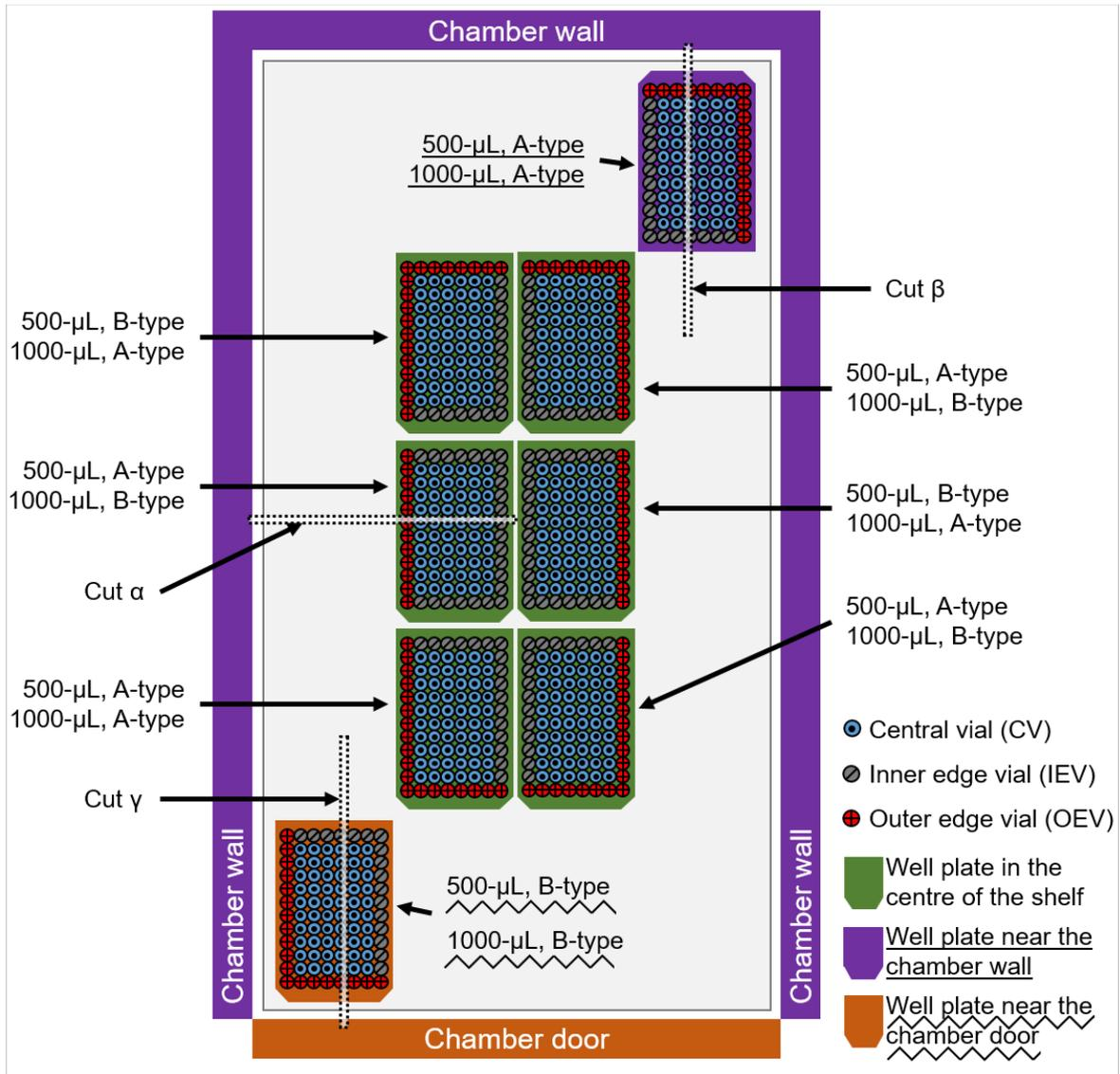
Figure 4.3-1 – Arrangement of the well plates on the freeze dryer shelf for tests (not in scale, view from the top). Dotted rectangles (cuts  $\alpha$ ,  $\beta$ , and  $\gamma$ ) denote sections of the system represented in the 3D models.
