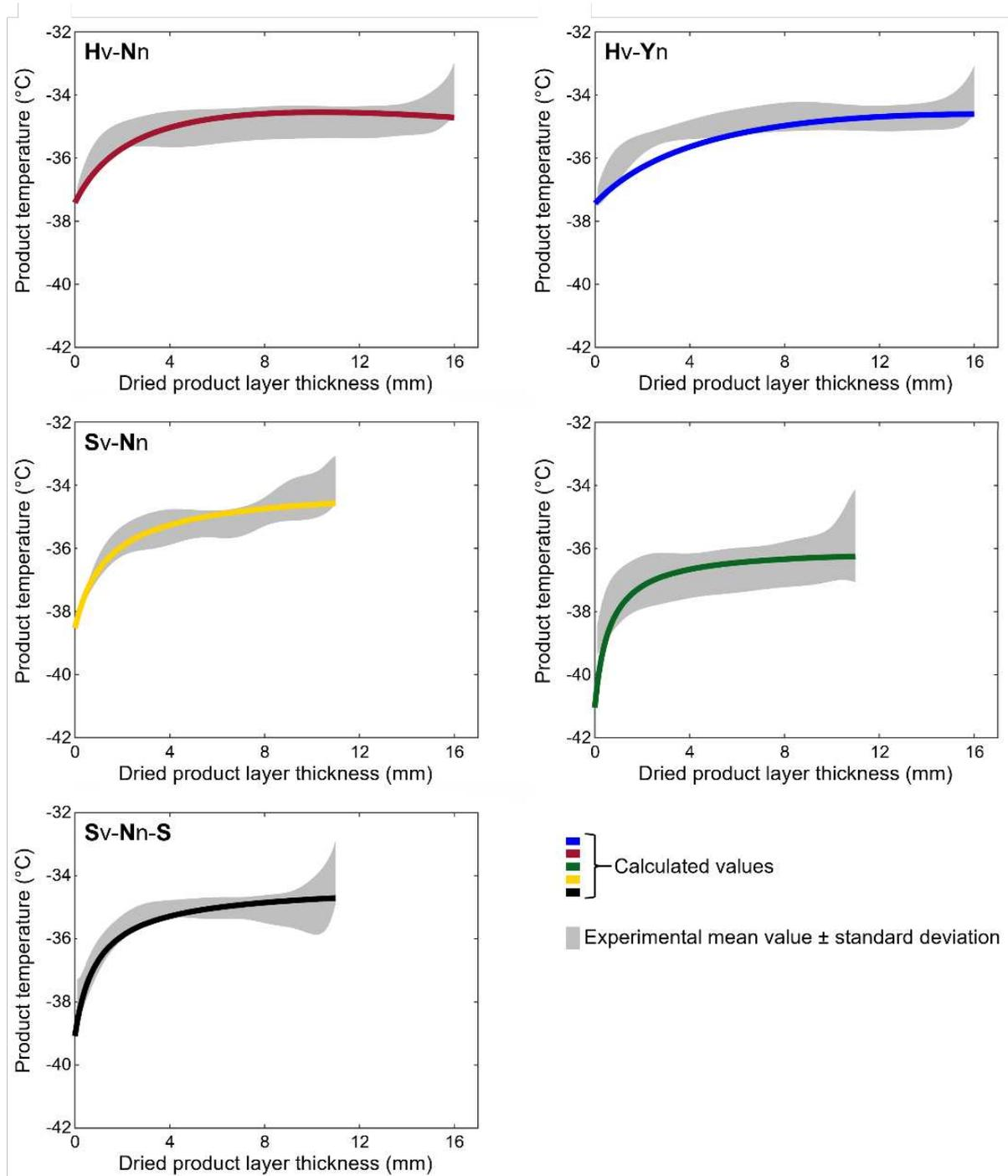
Figure 4.4-14 – Evolution of the product temperature with the dried product layer thickness ( $l_d$ ). Grey areas are the represent the mean values  $\pm$  standard deviations of the temperatures measured using the eight thermocouples, and coloured lines are the calculated temperatures using the area-normalised product resistance ( $R_p$ ) and Equation 4.4-1 to Equation 4.4-8. Hv-Nn, Hv-Yn, Sv-Nn, Sv-Yn, and Sv-Nn-S are the experimental conditions described in Table 4.4-1.
