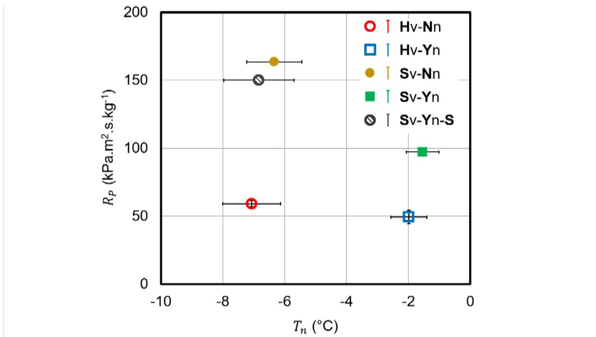
Figure 4.4-13 –  $R_p$  values at  $l_d = 5$  mm expressed as a function of the nucleation temperature ( $T_n$ ) determined using a thermal camera (Figure 4.4-6). Error bars in the  $R_p$ -axis are the  $R_p$  standard deviations of the three repetitions when using high-throughput vials (Figure 4.4-11). Error bars in the  $T_n$ -axis are the standard deviations (Figure 4.4-6). Hv-Nn, Hv-Yn, Sv-Nn, Sv-Yn, and Sv-Nn-S are the experimental conditions described in Table 4.4-1.
