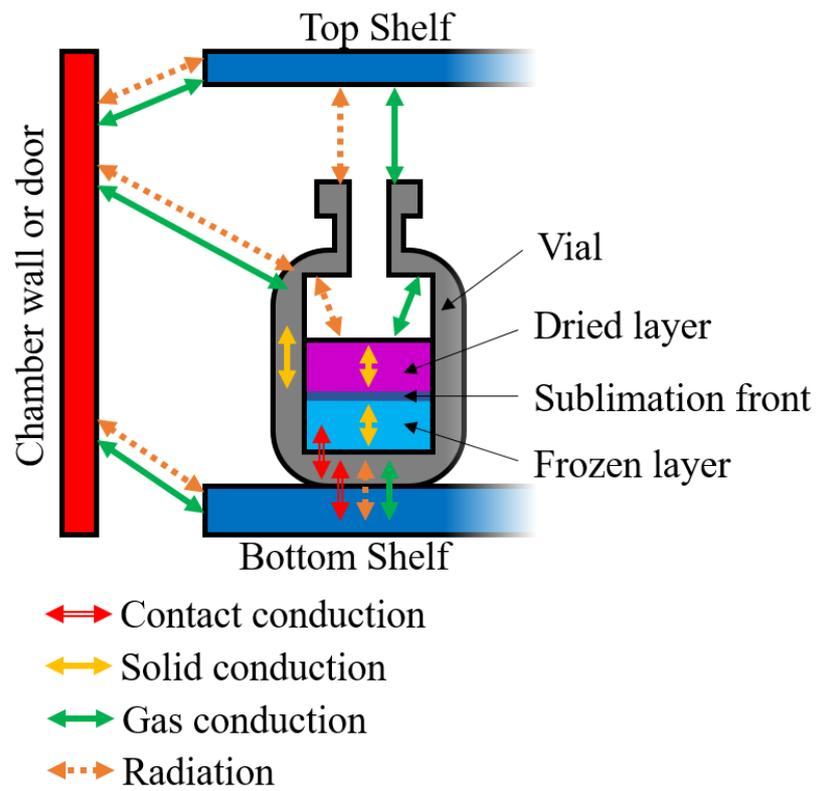
Figure 2.2-1 – Main heat transfer mechanisms (radiation and conduction) between bodies for a serum vial placed directly on the freeze dryer's shelf (adapted from Pikal, 2000).
