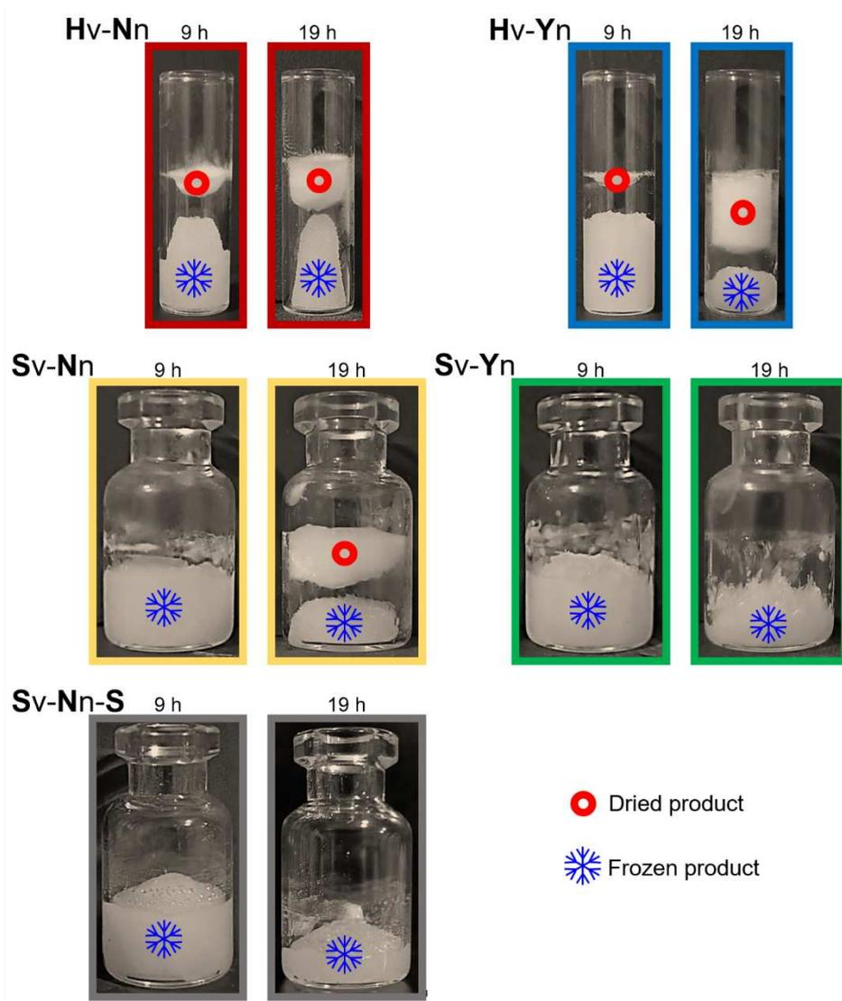
Figure 4.4-9 – Pictures of vials at intermediate points of primary drying taken after 9 or 19 hours of freeze-drying. Hv-Nn, Hv-Yn, Sv-Nn, Sv-Yn, and Sv-Nn-S are the experimental conditions described in Table 4.4-1.
