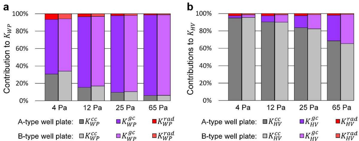
Figure 4.1-5 – Relative contributions of the heat transfer coefficients by contact conduction ( $K_{WP}^{cc}$ ,  $K_{HV}^{cc}$ ), conduction through the gas ( $K_{WP}^{gc}$ ,  $K_{HV}^{gc}$ ), and radiation ( $K_{WP}^{rad}$ ,  $K_{HV}^{rad}$ ) as percentages of the total heat transfer coefficients: (a) between shelf and wall plate ( $K_{WP}$ ), and (b) between wall plate and vial ( $K_{HV}$ ).  $K_{HV}$  values for 500- $\mu$ L vials.
