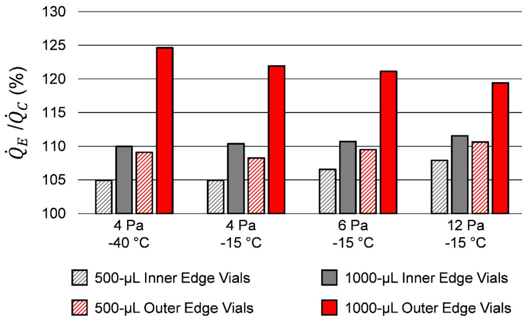
Figure 4.2-6 – Ratio (%) of  $\dot{Q}_E$  to  $\dot{Q}_C$  ( $= [\dot{Q}_E / \dot{Q}_C] \times 100\%$ ). Results were obtained using the distilled water model at different shelf temperatures (-40 and -15 °C) and chamber pressures (4, 6 and 12 Pa). Vial positions refer to those shown in Figure 4.2-2.
