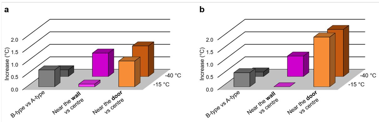
Figure 4.3-8 – Product temperature increase due to: (i) a B-type well plate instead of an A-type well plate (both in the centre of the shelf), (ii) placing the A-type well plate near the chamber wall instead of the centre of the shelf, (iii) placing the B-type well plate near the chamber door instead of the centre of the shelf. Results at chamber pressure 4 Pa.
