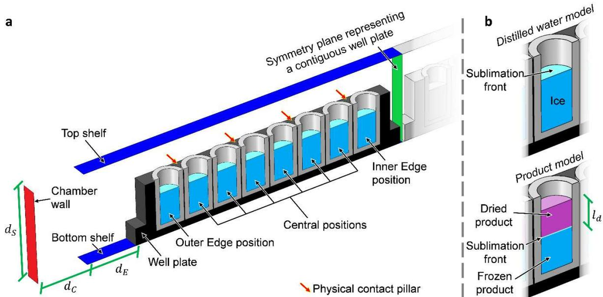
Figure 4.2-2 – Model geometry (not in scale) for 500- $\mu$ L vials in well plates. (a) Overall view, with only the vials closer to the chamber wall represented for clarity. (b) Detail of the vial and its content for distilled water and product models.  $d_s$  is the vertical distance separating shelves,  $d_c$  is the distance between the shelf and the chamber wall,  $d_E$  is the distance between the edge of the shelf and the well plate, and  $l_d$  is the dried product layer thickness.
