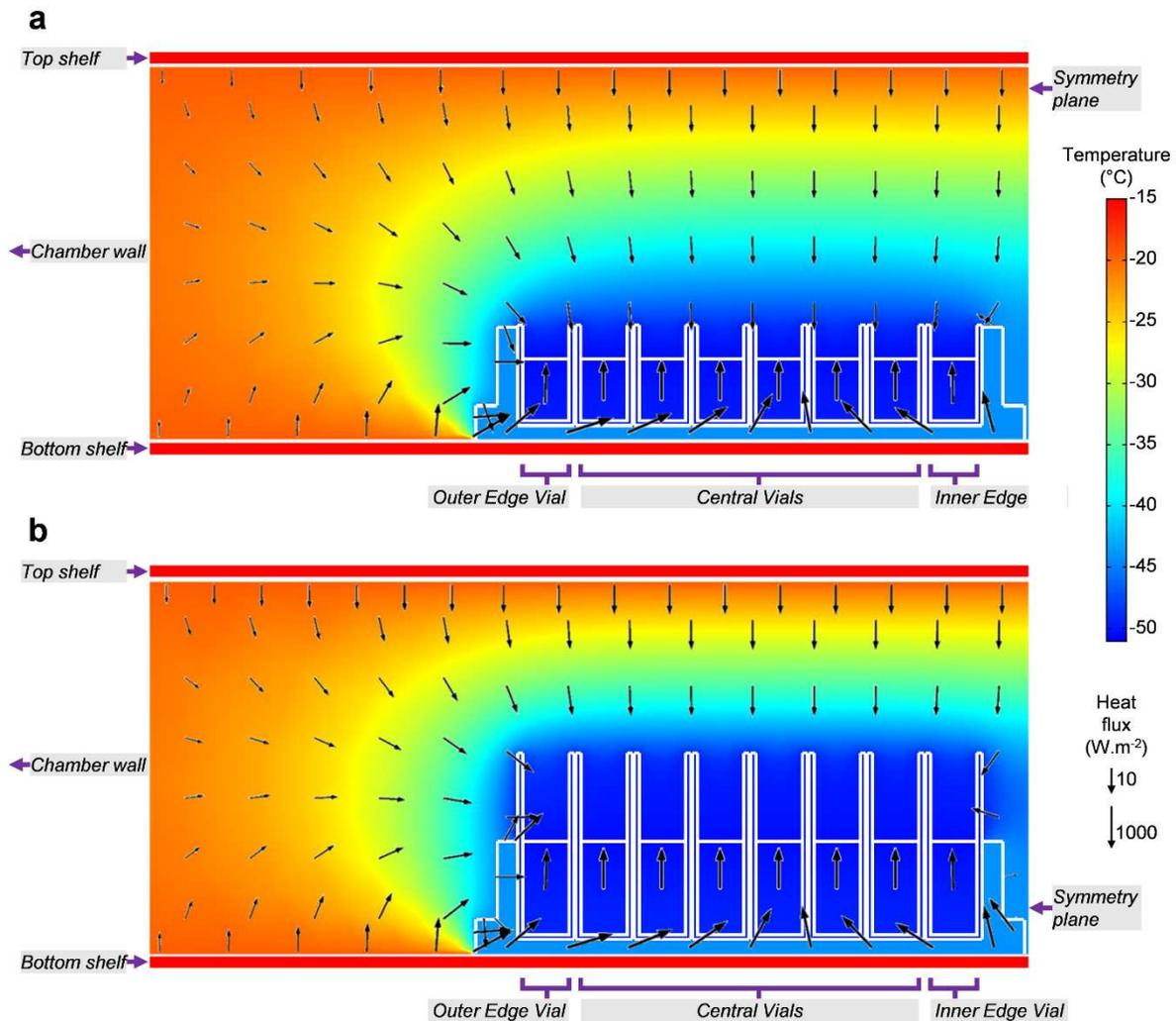
Figure 4.2-7 – Temperature profiles and heat fluxes obtained with the distilled water model for (a) 500-µL vials and (b) 1000-µL vials. Temperatures are represented as colour maps. Heat fluxes through the loose gas, vials and frozen product layers are represented as arrows whose lengths indicate their module on a logarithmic scale. Calculations were performed at a shelf temperature of -15 °C and a chamber pressure of 4 Pa.
