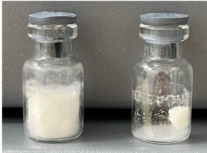
Figure 2.1-5 – Observation of product collapse. The left vial has an acceptable appearance; the right vial does not have an acceptable appearance (collapsed).
