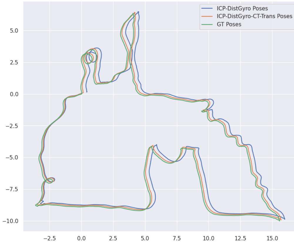
Figure 5.6: ICP-DistGyro (Blue), ICP-DistGyro-CT-Trans (Orange) and ground truth poses (Green). Dataset HILTI-2022, exp06
