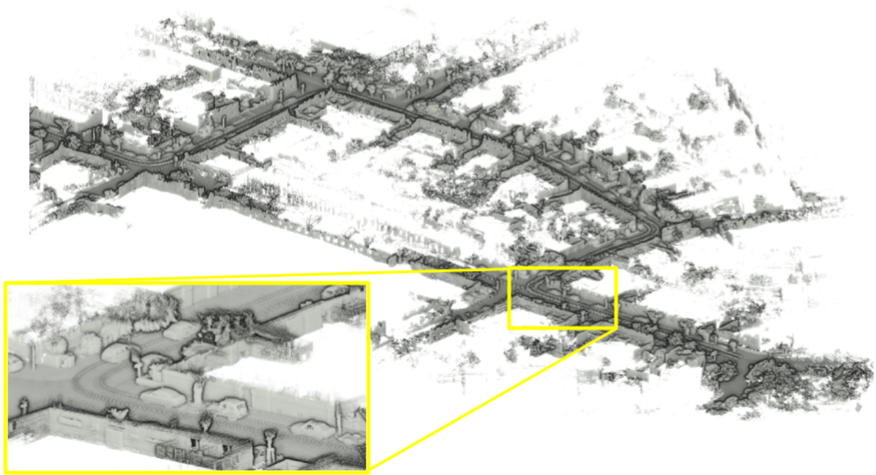
(a) Aggregated point cloud frames, using CT-ICP's trajectory on sequence 00 of the KITTI dataset.
