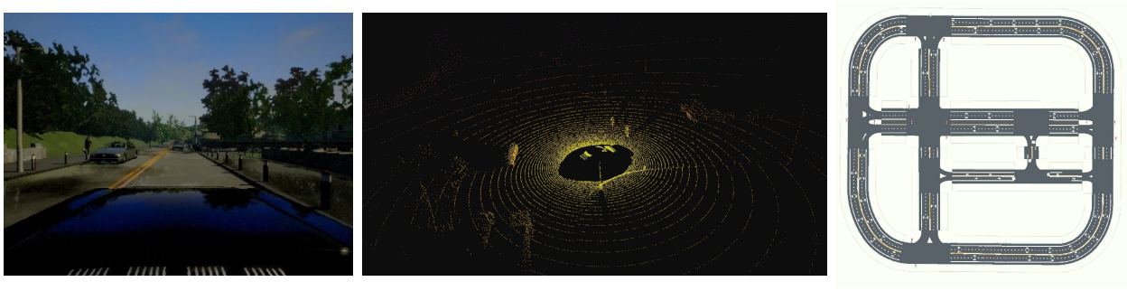
Figure 2.3: Images describing the sensor output of the CARLA dataset. Left: image from a simulated photorealistic RGB sensor. Middle: a sample LiDAR frame simulated with the engine. Right: the road layout of the map Town10.
