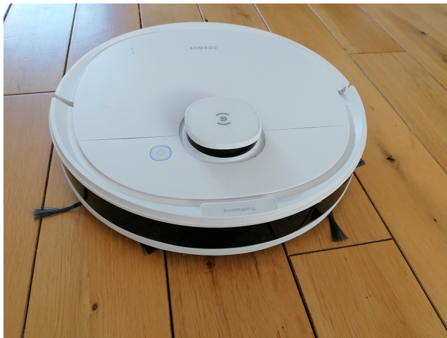
Figure 1.3: Vacuum Cleaner Robot, possesses a 2D LiDAR which maps to establish the optimal trajectory to clean it.
