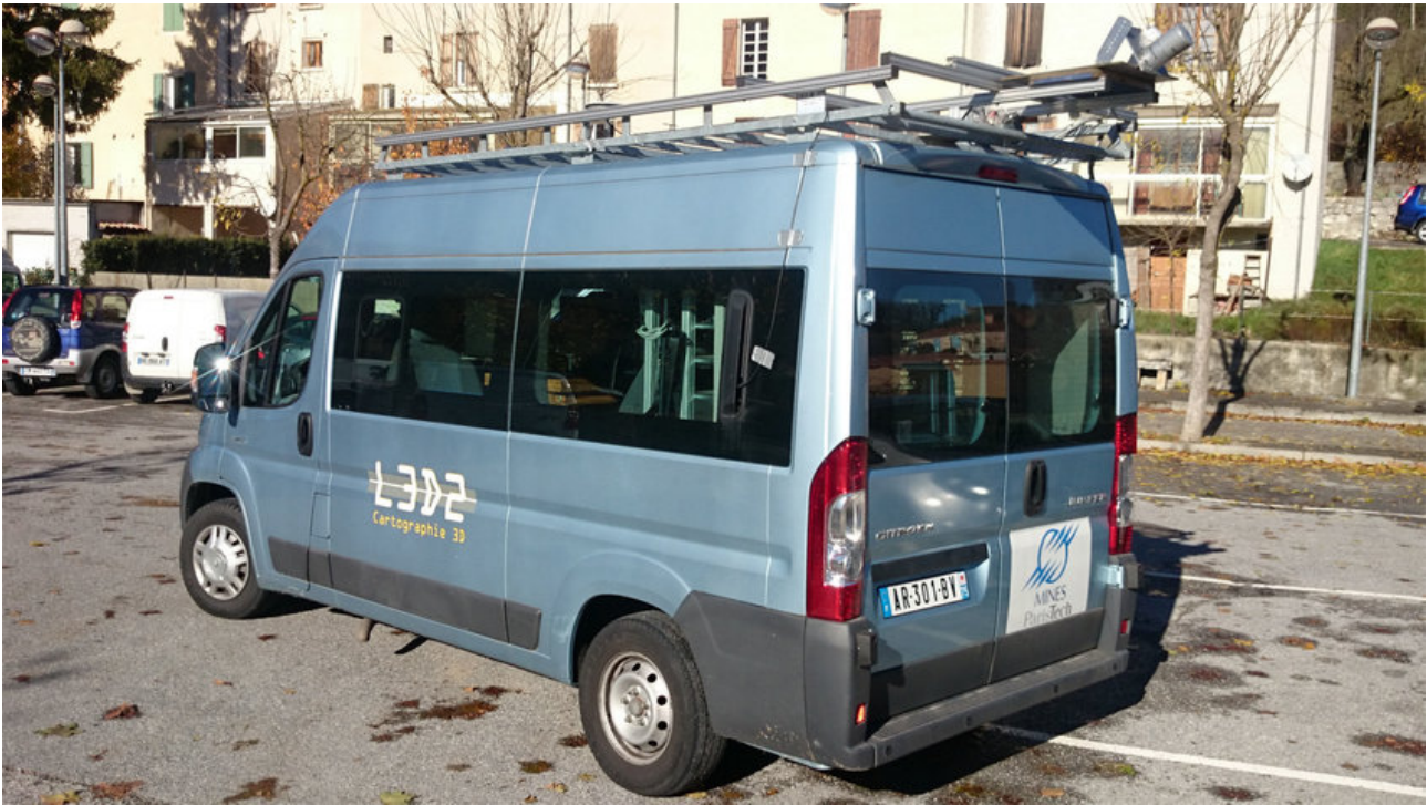
Figure 1.4: L3D2 acquisition platform constructed by the CAOR laboratory of MINES Paris-PSL. This platform relies on a costly industrial-grade GPS-INSS unit to construct a very accurate trajectory.
