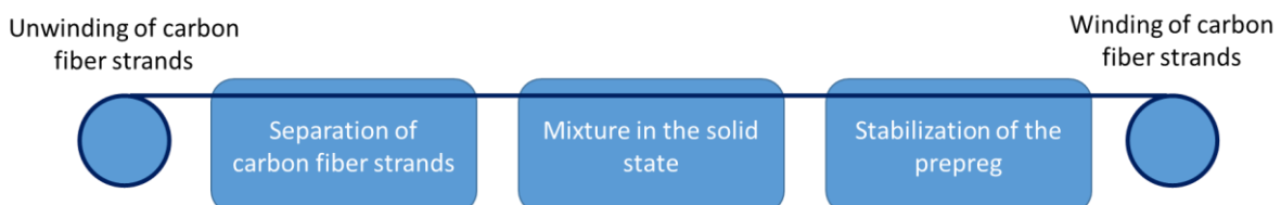
Figure I-3 : Scheme of CFRTP prepreg manufacturing process, adapted from [37]
