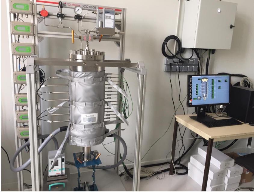
FIGURE 1.7 – Overview of the laboratory storage pilot and its components.
