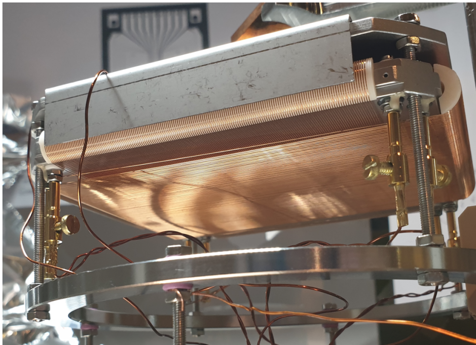
(b) Delay lines below the MCP
