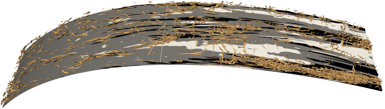
Figure 5.15: Isosurfaces of the tangential velocity fluctuation u'_s for -0.09c_{in} (black) and 0.09c_{in} (white), along with the Q-criterion (light brown), at the same instant as figure 5.14 from the LE to s/ch \approx 3.5\% .
