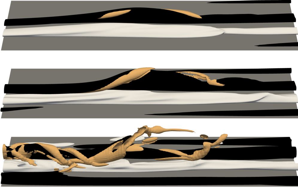
Figure 4.25: Observation of a sinuous-like breakdown in the high L_f -low T_u case at three successive times. Isosurfaces of the streamwise velocity fluctuations: u' = 0.16U_\infty (white), -0.16U_\infty (black). Isosurfaces of the Q-criterion are also depicted in light brown.
