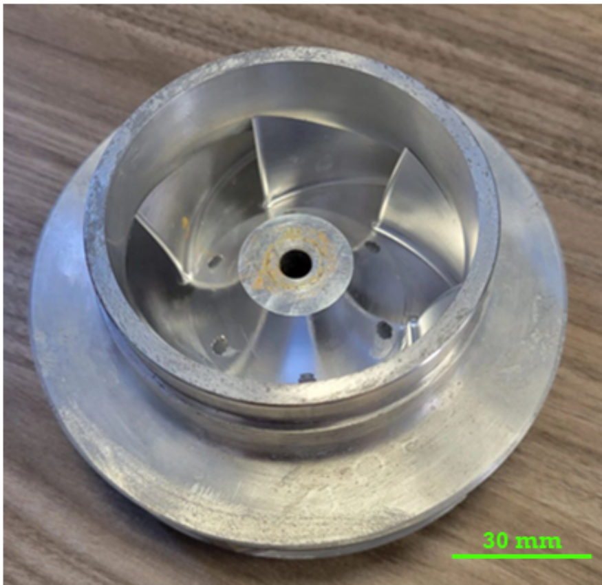
FIGURE 3.1 – Primary aluminium centrifugal impeller
