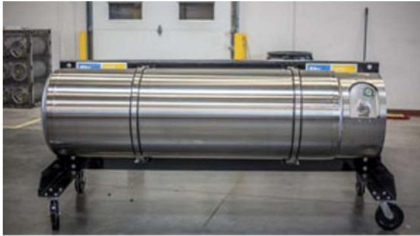
Figure 2. a) An image of Small Scale tank that contains bio-LNG as industrial fuel in Valenton, France [13]. b) A picture of SS storage container of a truck fuelled with LNG [14].
