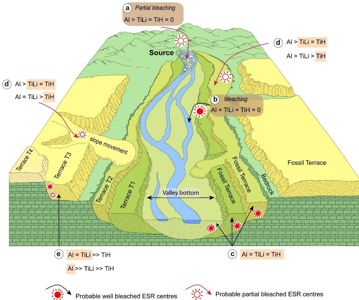
Figure 3.2. Paramagnetic centres intensity expected in a fluvial environment. Orange rectangles represents the preferable centre to give an ESR age. (a) In erosion zone, the Ti-centre can bleach very quickly but Al-centre are not completely bleached. (b) In river bed, all three centres are completely bleached. (c) In the fossil terrace, all three centres have a signal that increase over time. (d) In case of grain remobilisation from an older sediment or when transport has been insufficient, exposure to light was not sufficient for the Al-centre to be fully bleached but the Ti-centre can be bleached. (e) In old fossil terraces, the bleaching cycle of the eroded grains will begin again and can be complete or not.
