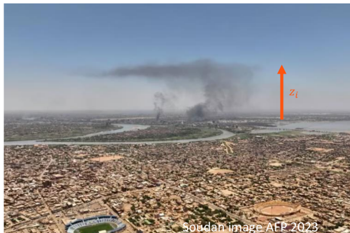
Figure 1.14: Smoke plume capped by a stable layer (at the altitude z_i ) and rotating rightward due to Coriolis effects in the Ekman layer.
