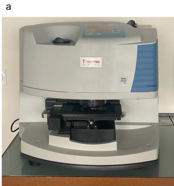
FIGURE 18A – PHOTOGRAPH OF THE NICOLET iN10 USED FOR MICROPLASTIC ANALYSIS; B – PHOTOGRAPH OF THE NICOLET iS5 USED FOR THE CHARACTERIZATION OF MACROLITTER.
