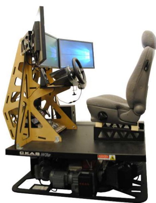
(a) VR Driving Sim Setup
