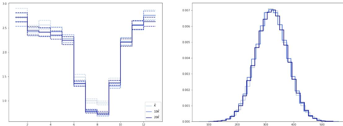
Figure 1.17: Average payoffs for different values of  $K \in \{\hat{K}, 10\hat{K}, 20\hat{K}\}$  (left), HDD distribution distribution starting from  $HDD_{strike}$  (right) for a derivative on the month of January 2019, forecasted 30 days ahead and based on 50,000 Monte Carlo simulations (right).  $HDD_{strike}$  is kept at 90% empirical quantile of  $K = \hat{K}$  for all simulations.
