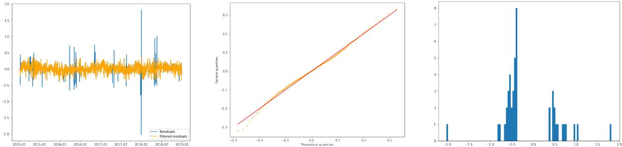
Figure 2.3: Jump filtering method as described by Carlea and Figueroa [49] (left). Filtered continuous residuals qqplot against a normal distribution (center). Histogram of jumps (right).
