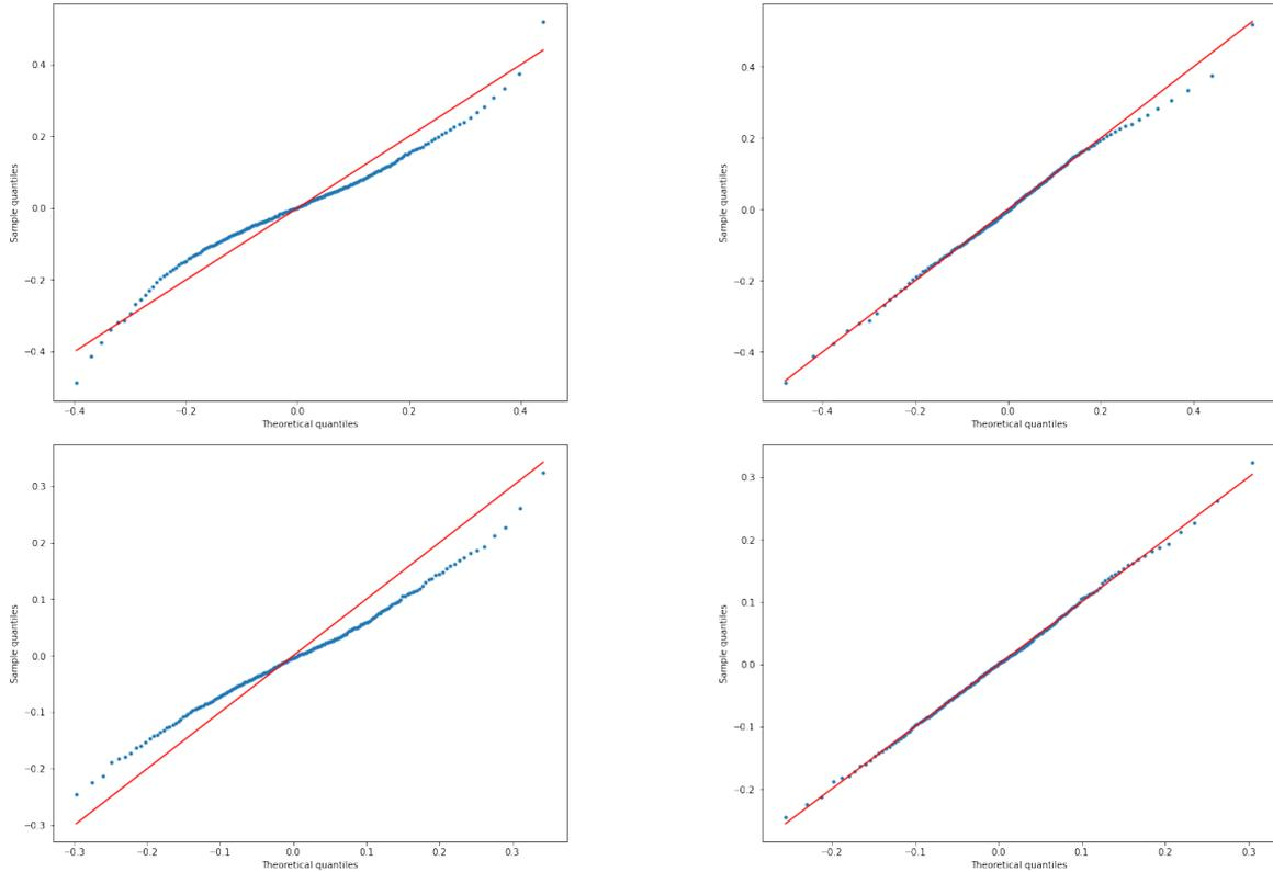
Figure 2.2: Quantile quantile plots for residuals of Regression (2.3) compared with a theoretical quantiles of a normal distribution (left) and of a normal inverse gaussian distribution (right) for French energy (first row) and North Italian Energy (second row).
