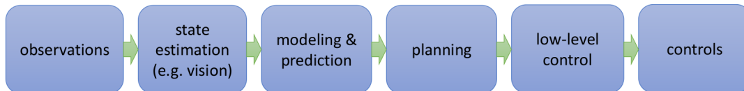
FIGURE 1.3: Classic robotic control pipeline (source: Levine, Fa2019 )
