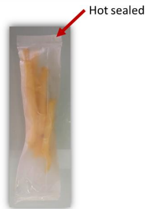
Figure IV.11: Hot sealed film of PHBV/PBSA + 0.1phr DCP filled with frozen French fries
