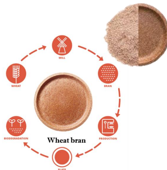
Figure VI.14: Schematic representation of BIOTREM technology, image reproduced from (BIOTREM., 2016)
