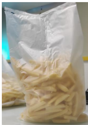
Figure V.7: Hot sealed film of PHBV/PBSA/ATBC 63/27/10 + 0.2 phr luperox filled with 625 g of frozen French fries
