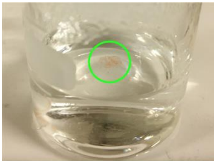
Figure 2.2 Polymeric membrane formation using 0.5 mg/ml Poly(NIPAM-co-SPMA) in water.
