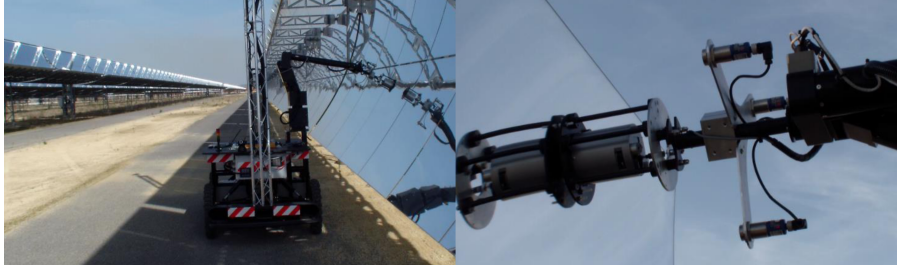
FIGURE 2.21 – Mirror reflectivity measurement at VALLLE energy plant by MAINBOT adopted from[64]
