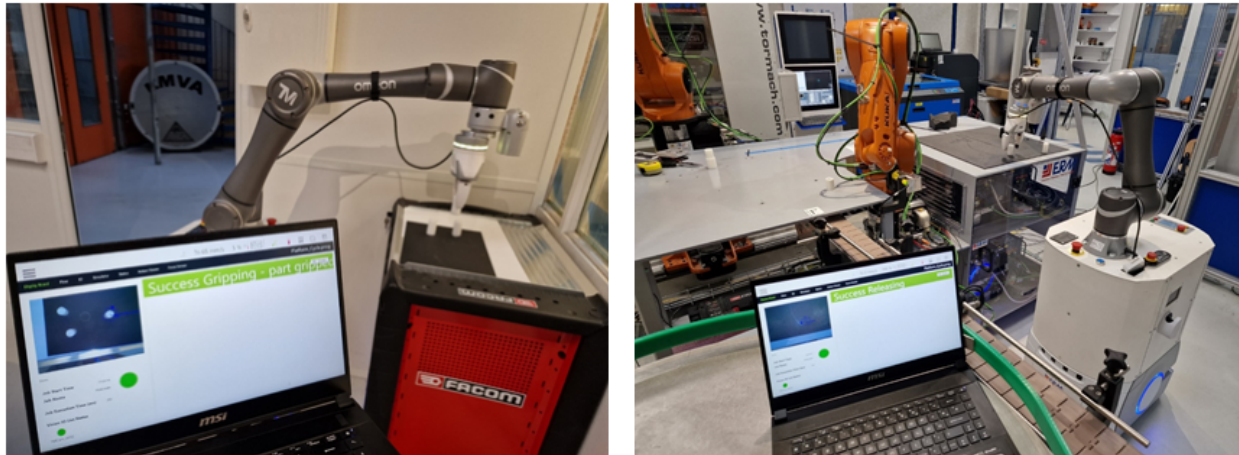
FIGURE 4.8 – Vision-guided picking operation of raw parts (left) and vision-guided placing operation of raw parts (right)
