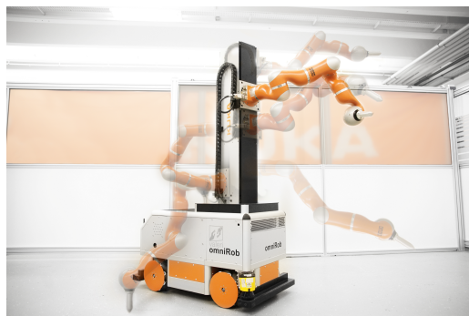
FIGURE 2.23 – KUKA VALERI mobile manipulator adopted from [73]
