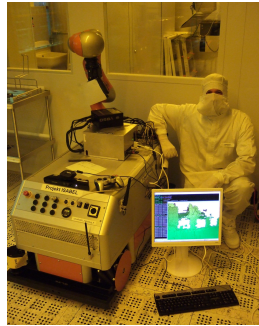
FIGURE 2.20 – ISABEL MM implementation for wafer box pick and place in clean room adopted from [63]
