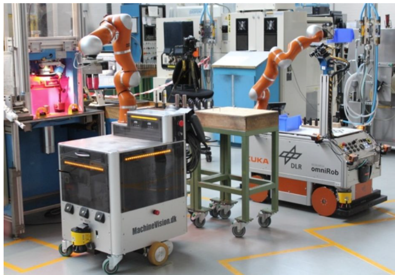
FIGURE 2.13 – Little Helper 3 from Aalborg University (Left) omniRob from KUKA (Right)
