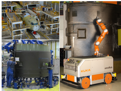
FIGURE 2.22 – The use of MM in aerospace production system of Airbus Defence Space adopted from [68]
