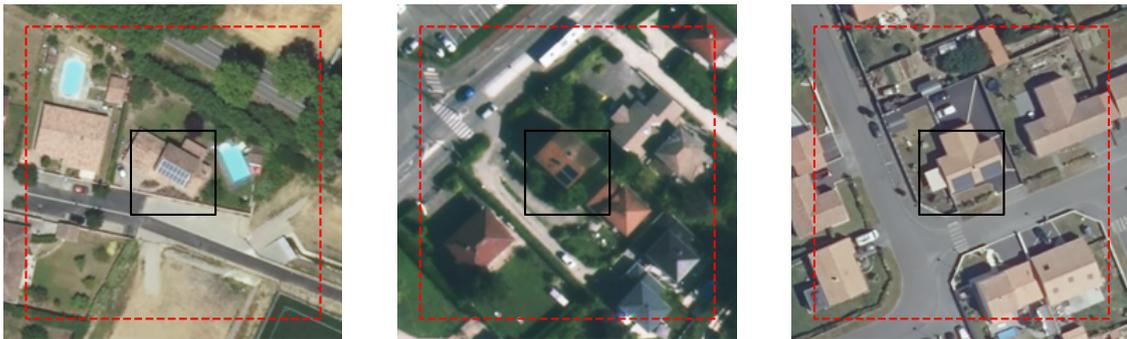
Figure 4.6 – Illustration of the cropping of thumbnails of a size of  $224 \times 224$  pixels from the raw BDAPPV image with a size of  $400 \times 400$  pixels to simulate various locations of the PV panel on the image. The black square is always included in the smaller thumbnails, the red dashed lines indicate the boundaries of the thumbnails, such that this black square is contained in the thumbnail.
