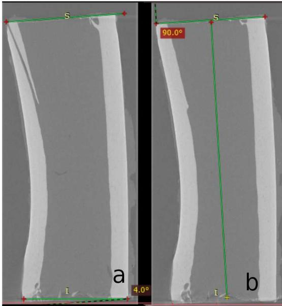
Figure 68: a) 4° Misalignment (note a blood vessel entering the bone). b) alignment with the longitudinal axis, specimen Nr.3, 2nd group.
