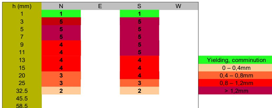
Figure 52: Example of pattern of rupture obtained from MicroCT analysis. Colours relate to the size of crack for the pattern of damage.
