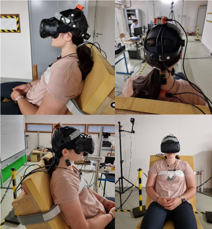
Figure 38 : Participant outfitted with physiological sensors and HMD sitting on the SLED
