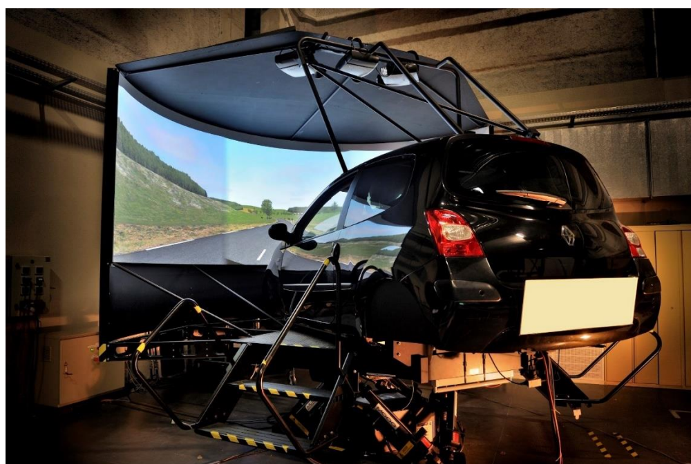
Figure 16: Renault Twingo skeleton mounted on the Moog 6DOF200E motion system platform (Also known as SAAM)
