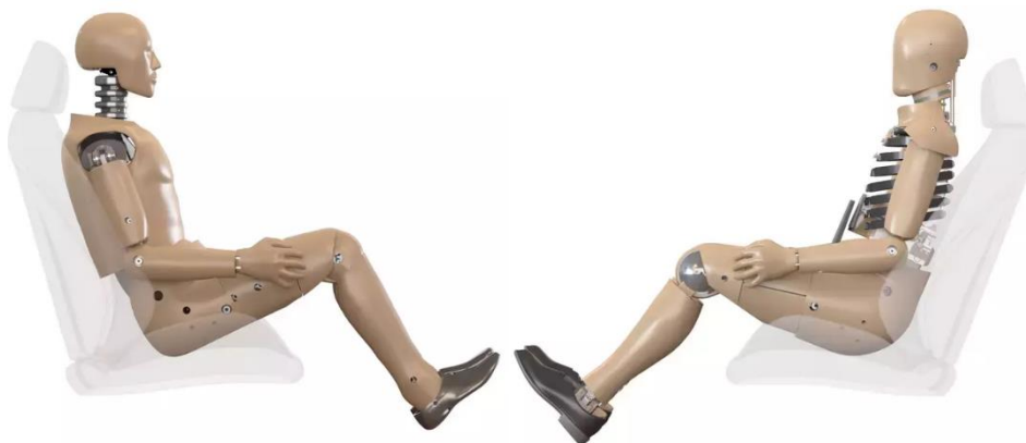
Figure 6: Hybrid III crash test dummy (left); THOR crash test dummy (right) (Humanetics 2024)
