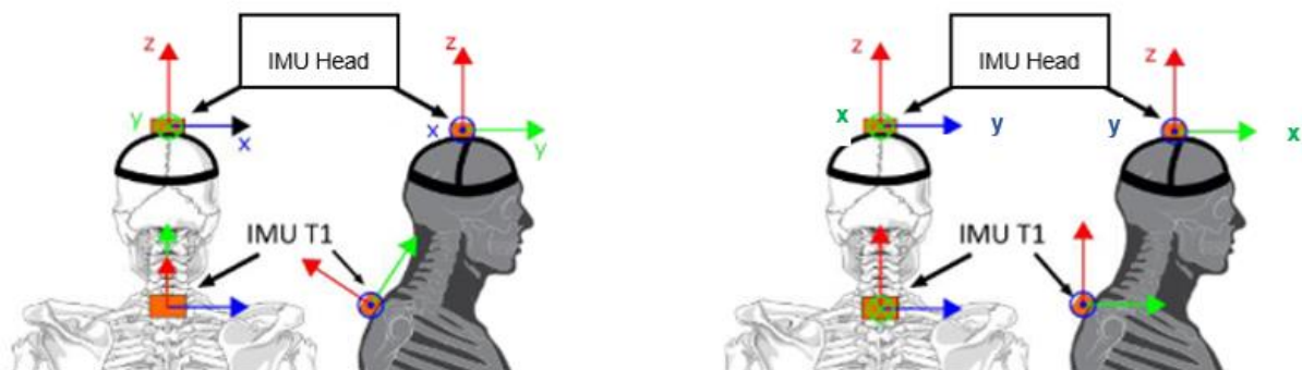
Figure 49: Alignment of IMU reference frames, Before Alignment (Left); After Alignment (Right), adapted from Patrick J. Lynch & C. Carl Jaffe
