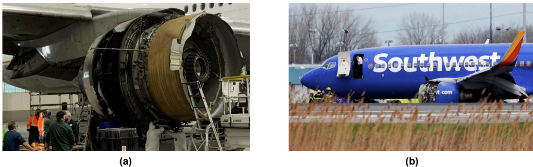
Figure 1.1: In (a), the inspection of a non-crashed Boeing 777-200 engine which suffered from turbine blade fatigue failure on United Airlines Flight 328, on Feb. 20, 2021. In (b), a crashed Boeing 737-7H4 which suffered from turbine blade fatigue failure and killed a passenger on Southwest Airlines Flight 1380, on Apr. 17, 2018.
