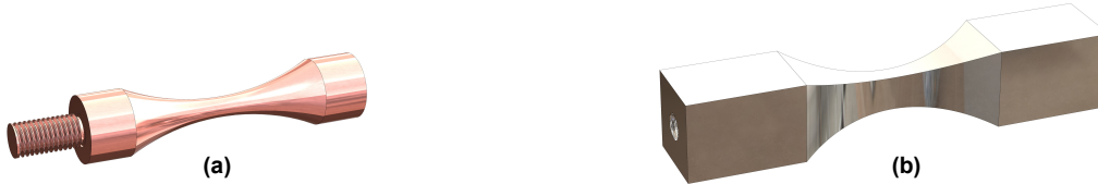
Figure 1.19: In (a) and (b), a hourglass and a rectangular ultrasonic fatigue specimen, respectively.
