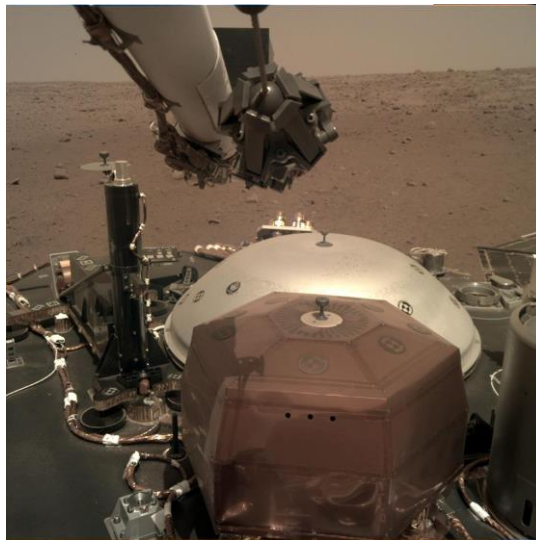
Figure 1-9. Instrument payload on the landing deck. From left to right, the HP 3 probe, the thermal shield of SEIS and the SEIS instrument (red)
