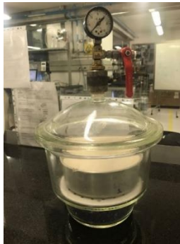
Figure 5-27. Vacuum chamber to preserve the soil dry as the material cools down.
