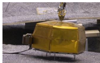
Figure 3-2. Testing of the SEIS instrument on Earth. (SEIS: Insight’s Seismic Experiment for Internal Structure of Mars (2019))
