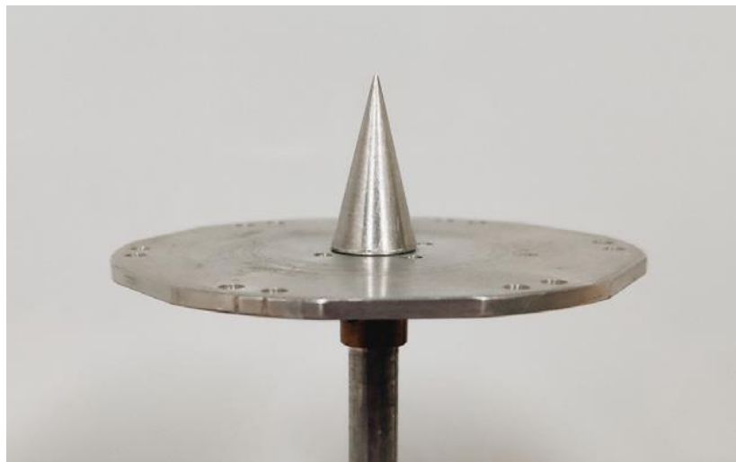
Figure 3-22. The shape of the SEIS foot. The conical spike has a maximum diameter of 10 mm.
