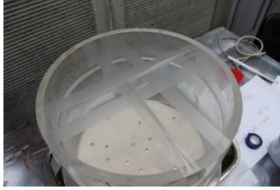
Figure 2-3. Tape used to ensure the central position of the funnel during pluviation.
