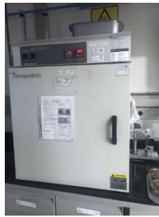
Figure 5-26. The material was dried in an oven for two days before the sample was prepared.
