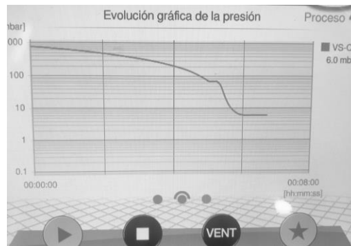
Figure 5-31. The desired pressure is applied in two steps to avoid disturbing the sample.
