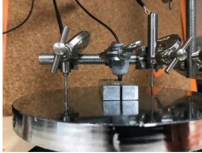
Figure 3-5. Testing process of displacement sensors. The non-contact Eddy sensor is seen in the middle.
