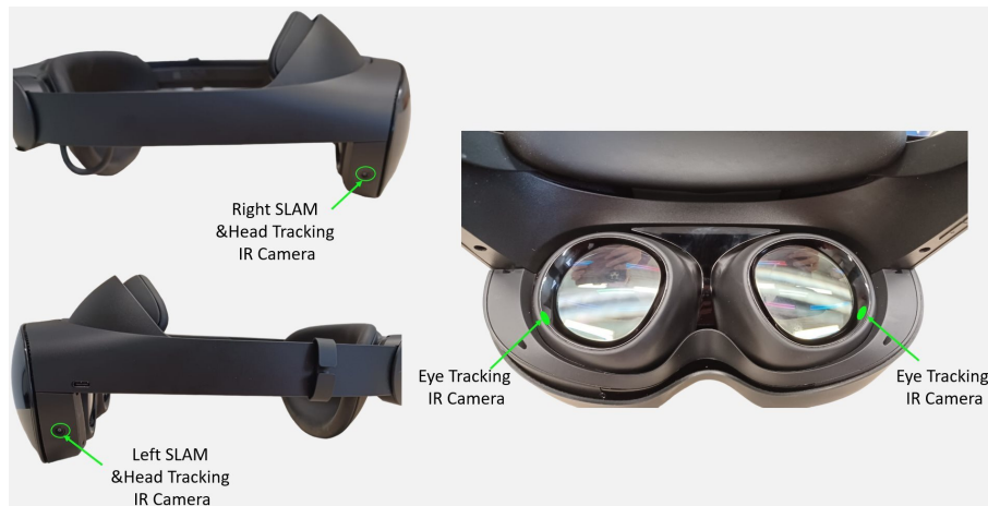
Figure 4.21: The Meta Quest Pro headset collects behavioral measurements, including eye-tracking and head-tracking data. The Data TCP Client is a TCP client that connects to the core VR application to receive real-time behavioral and application data recordings.
