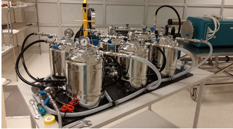
Figure 3.5: Filtration station. Picture taken in LULI2000 class-100 clean room.
