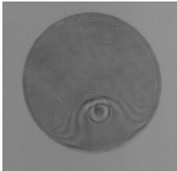
Figure 5.9: Spatial profile of the Stokes beam measured by a burn paper. Hard aperture of diameter 50 mm placed in the pump beam and uncentered. The hot spot location remains centered on the optical axis of the L_1 focusing lens.
