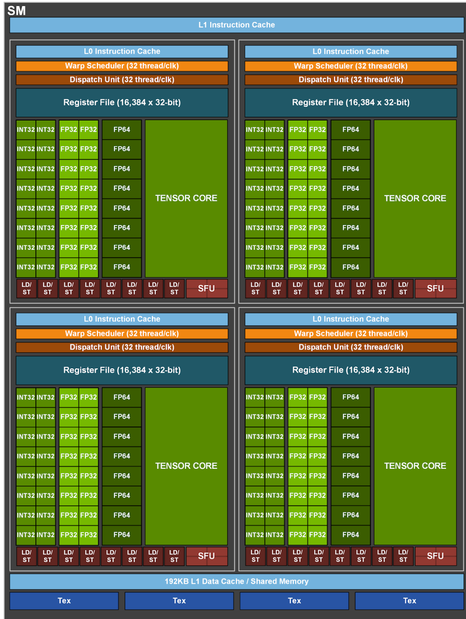
FIGURE 4.2 – Overview of a Streaming Multiprocessor (SM) of the NVIDIA Ampere GPU (A100) [NVIDIA, 2020] .
