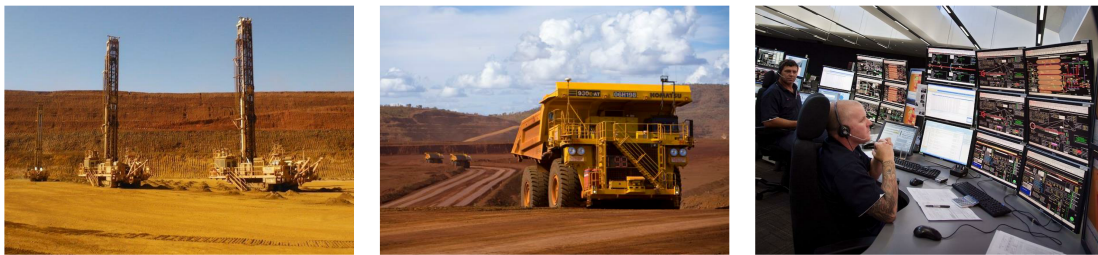
FIGURE 3: Example of machine-to-machine connection: Rio Tinto autonomous drilling system (left), haulage (center) and supervision room (right) [4].
