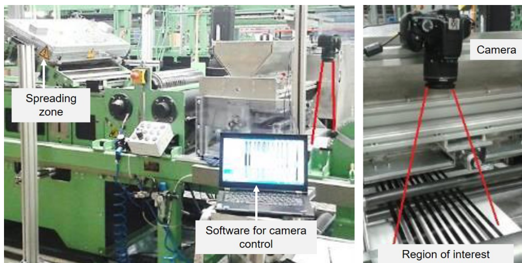
Fig. 3.11 Image recording setup for spread tow width measurement.
